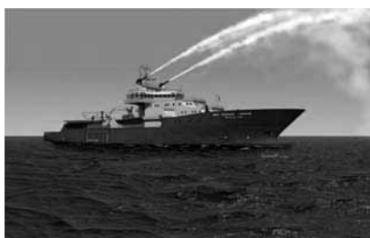
Figure 9 — UT527 Multi-field Standby Vessel demonstrating its fire fighting, pollution control and survivor recovery capabilities. Immediately noticeable are the capabilities for a medium size helicopter and dock/ramp for far interception or recovery boat
