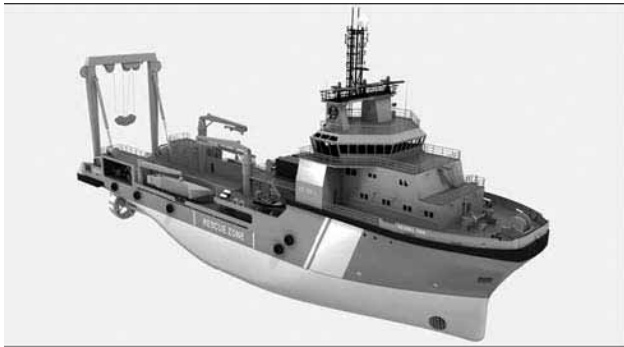
Figure 3 — UT-722L Emergency Towing and Pollution Control Vessel for Spain showing the very-large nozzled propellers necessary for such a very high bollard pull vessel.
