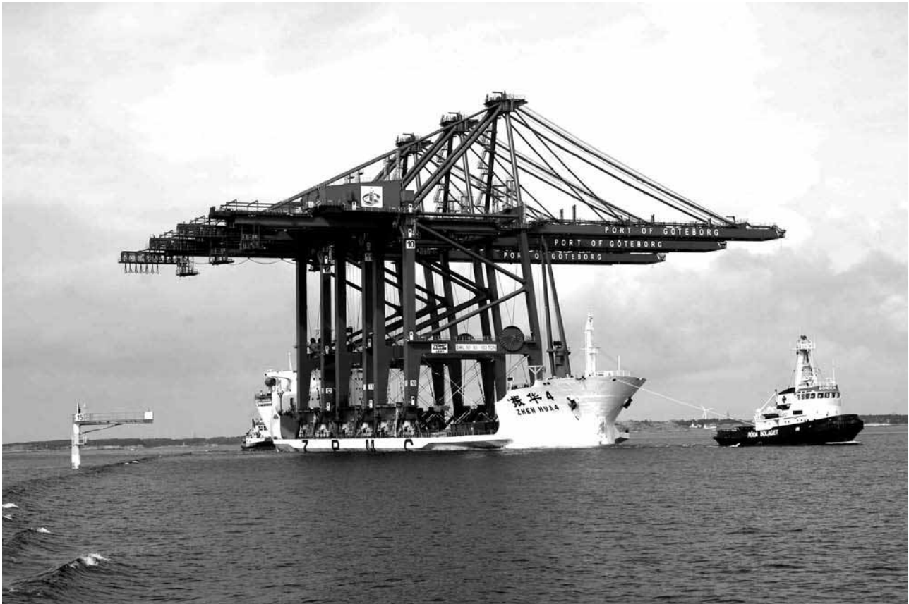
Three super-postpanamax container gantry cranes arriving at the Port of Göteborg, Sweden, in August. Similar new cranes have recently been delivered to Australian ports. The cargo is a reminder of the importance of careful stability calculations! The crane supplier, the Shanghai Zhenhua Port Machinery Company in China operates thirteen similar ships for delivery of its products worldwide (Photo courtesy Port of Göteborg)
