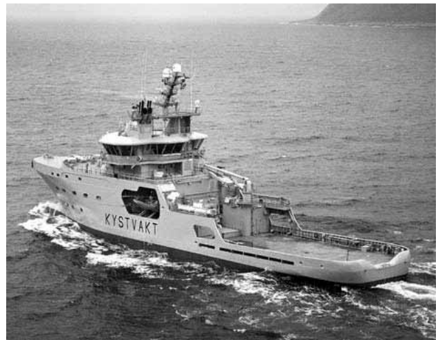
Figure 6 — UT512 Norwegian Coastguard Protection Vessel showing the extensive working deck aft
