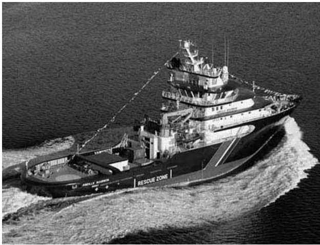
Figure 4 — The UT-515 Coastal Protection Vessel for France combined very high bollard pull with a high ship speed.
