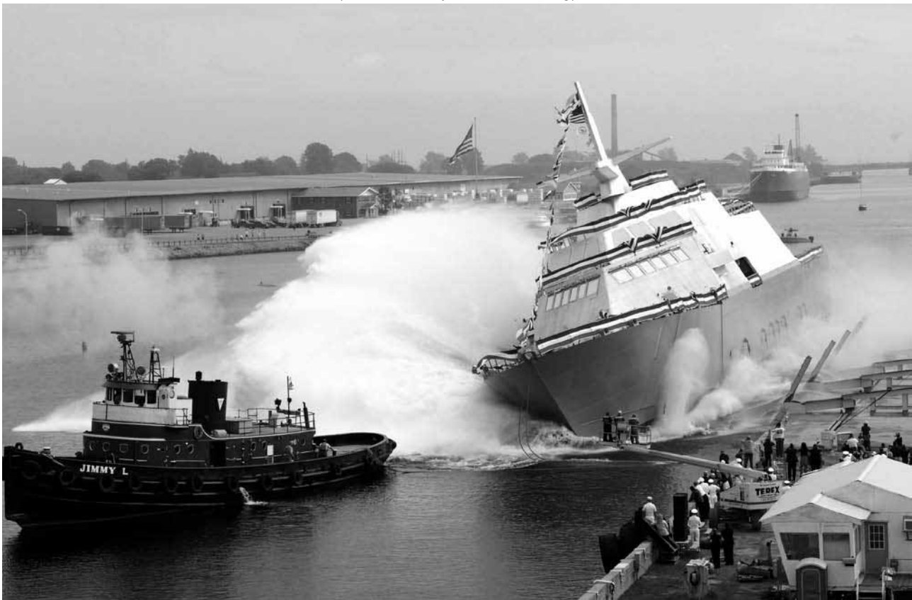
The first US Navy Littoral Combat Ship was launched in Marinette, Wisconsin on 23 September. Named Freedom , LCS 1 is the first of the two competing designs to be launched — the other is under construction by Austal USA. Freedom is a steel monohull design, 114.5 m long overall, with a designed top speed of over 40 knots (US Navy photograph)
