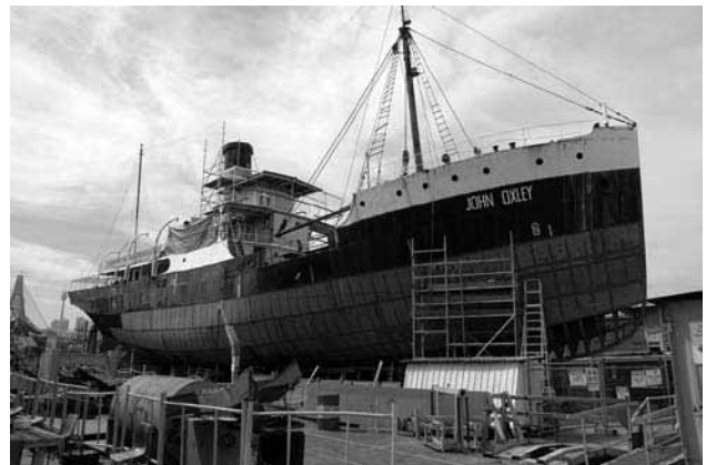
Considerable progress has been made replating the hull of John Oxley at the SHF shipyard in Rozelle Bay, Sydney (Photo John Jeremy)
