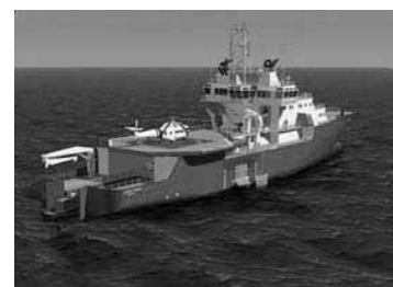
Figure 9 — UT527 Multi-field Standby Vessel demonstrating its fire fighting, pollution control and survivor recovery capabilities. Immediately noticeable are the capabilities for a medium size helicopter and dock/ramp for far interception or recovery boat
