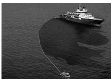
Figure 9 — UT527 Multi-field Standby Vessel demonstrating its fire fighting, pollution control and survivor recovery capabilities. Immediately noticeable are the capabilities for a medium size helicopter and dock/ramp for far interception or recovery boat
