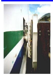
Fig 2 The Iron Sailor<sup>TM</sup> mounted forward on the port side of the Aratere in Wellington, NZ
