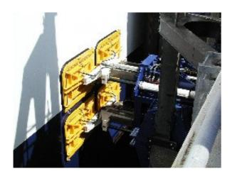
Fig 1- One of the 80 tonne Mooring System Ltd automated vacuum system which are installed for the Phase I development of the new Port of Dover
