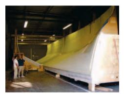
Figure 2: Hull Shell being assembled
