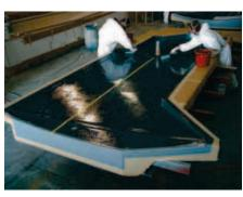
Figure 8: Strut Shell Mould
