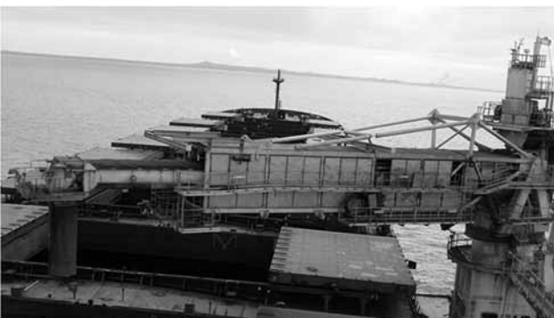
Conveyor system from FOTB onto the bulk carrier (Photo courtesy CSL Australia)
