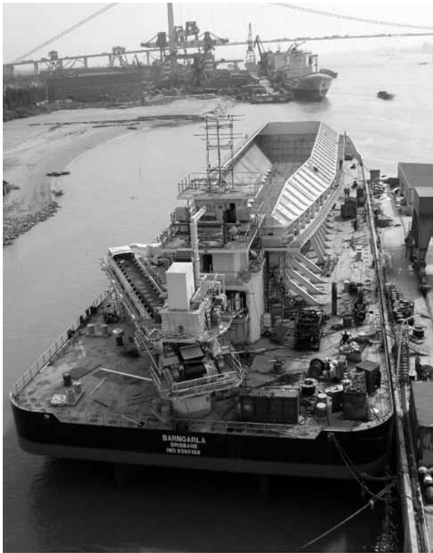
Self-unloading barge Bargarla fitting out in China, showing the hopper and conveyor for unloading onto the FOTB (Photo courtesy CSL Australia)
