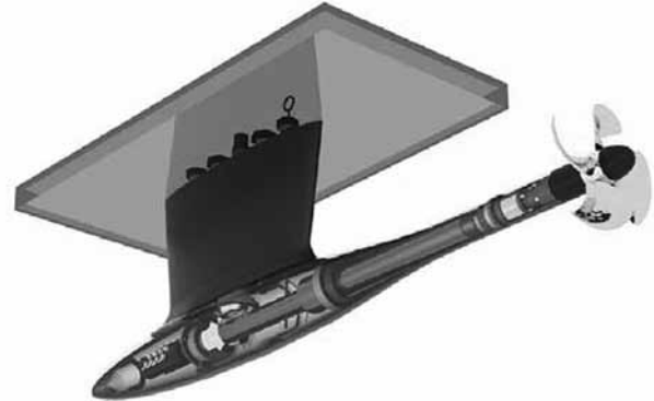
Figure 2: Propeller Dynamometer Schematic
