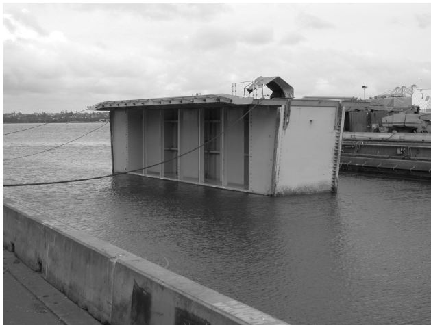
The dock gate during inclining—the gate's flotation tanks were ballasted to introduce a roll, and the upper gate cavity was used to stabilize the gate once it was on its side.
