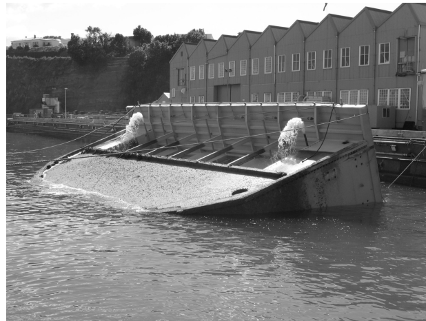
The dock gate during inclining—the gate's flotation tanks were ballasted to introduce a roll, and the upper gate cavity was used to stabilize the gate once it was on its side.
