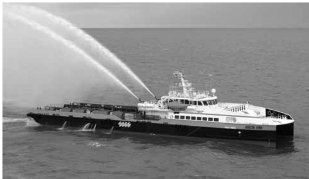
SEACOR Lynx testing fire monitors (Photo courtesy Incat Crowther)
