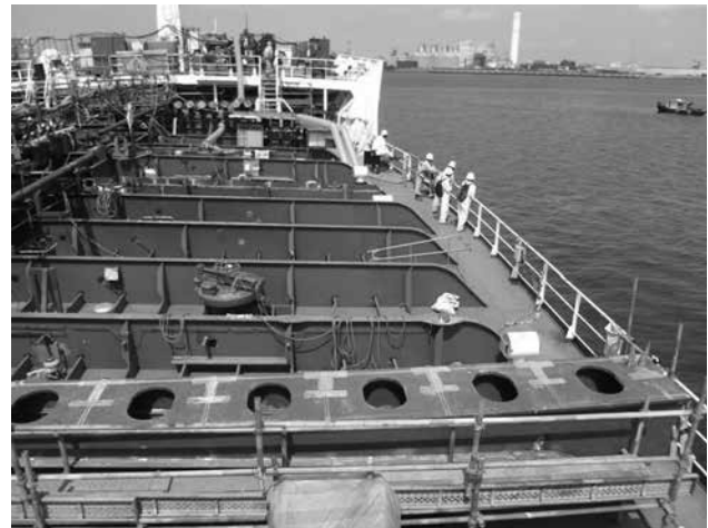
View of deck showing a plinth for raised-deck structure (bottom) (Photo courtesy ASO Marine Consultants)
