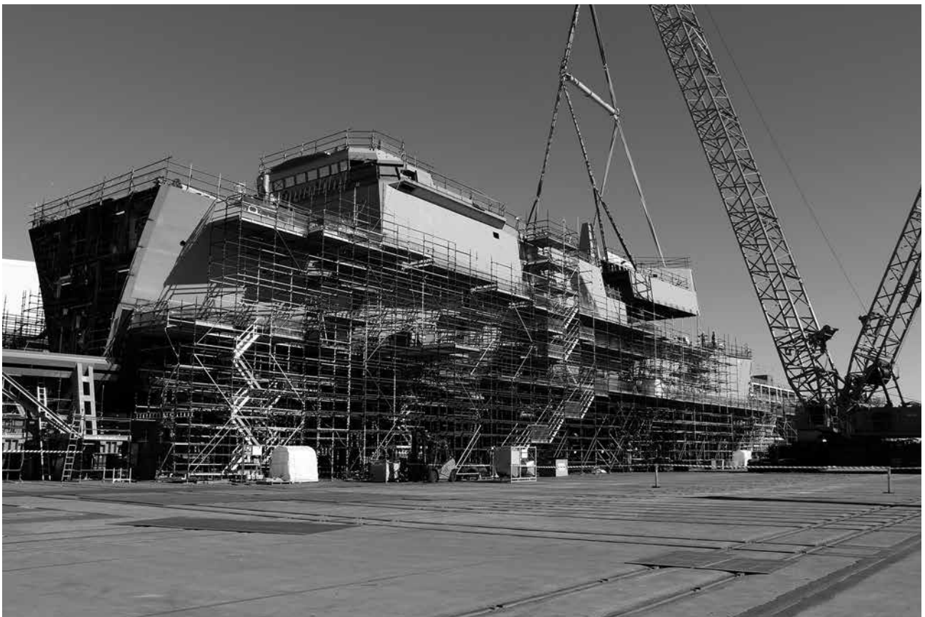
A 136 t superstructure block being erected on the future HMAS Hobart (Photo courtesy AWD Alliance)
