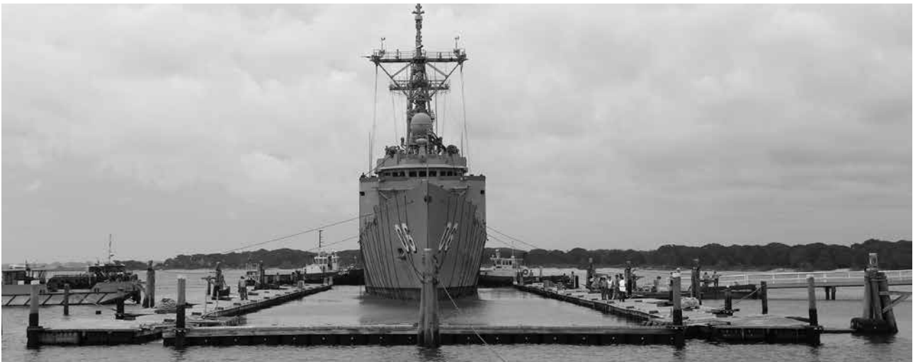
HMAS Newcastle entering the Magnetic Treatment Facility at Fleet Base West for a deperm in May in preparation for her deployment to the Middle East (RAN photograph)
