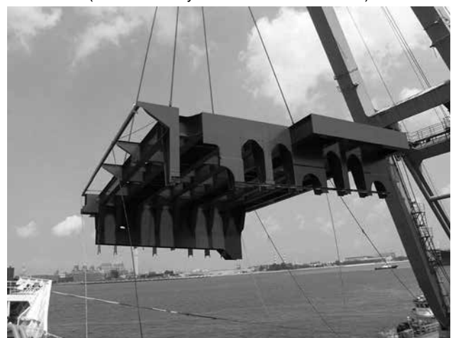
Raised-deck structure being lifted on board (Photo courtesy ASO Marine Consultants)
