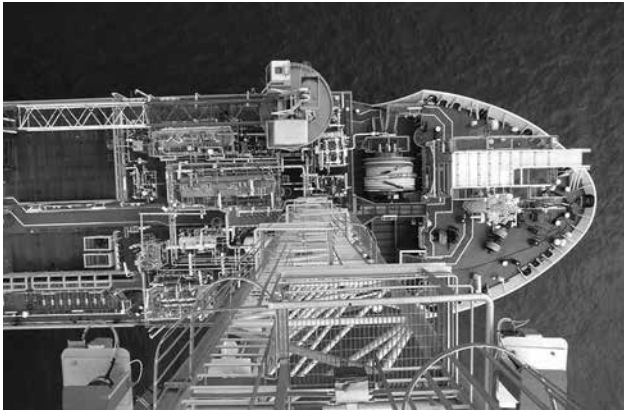
View from the top of the flare tower, showing the crane (left), hose reel (centre) and hawser chute (right) (Photo courtesy ASO Marine Consultants)
