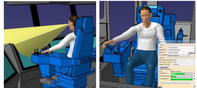
Figure 8: Ergonomic analysis on task specific postures (e.g. view, operating force)
