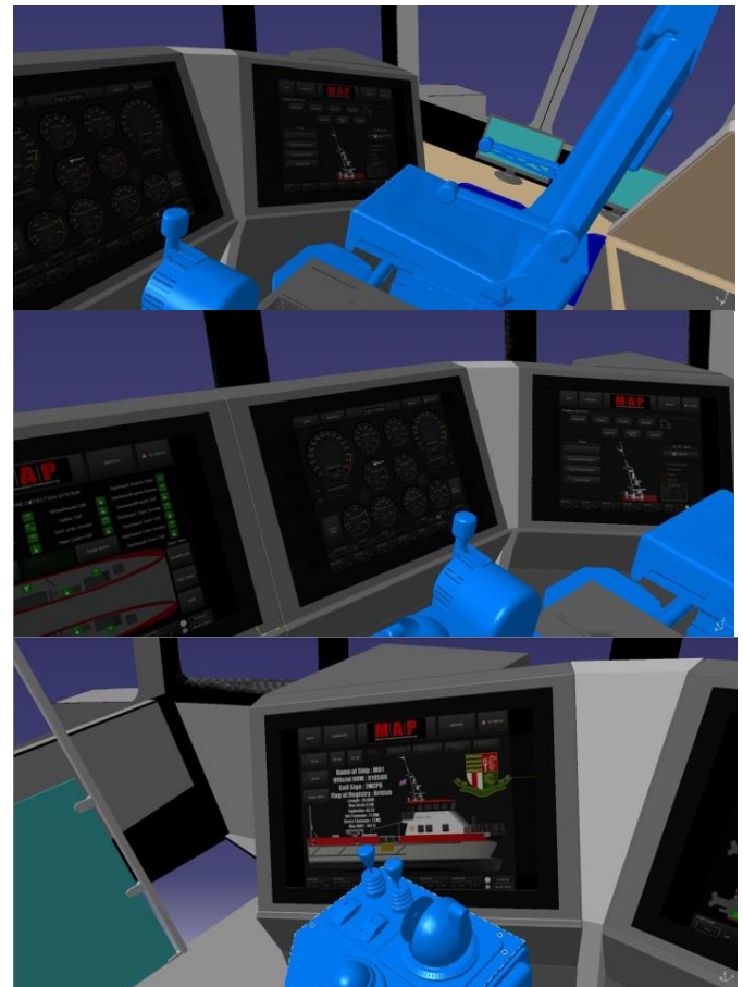
Figure 9: Vision through eyes of the manikin in operation posture (left, middle, right display)
