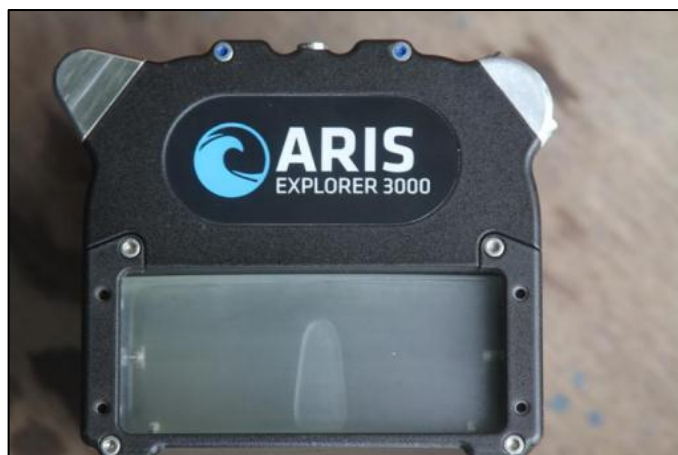
Figure 19 - The ARIS 3000 Sonar uses an Acoustic Lens to Facilitate Beam-Forming
