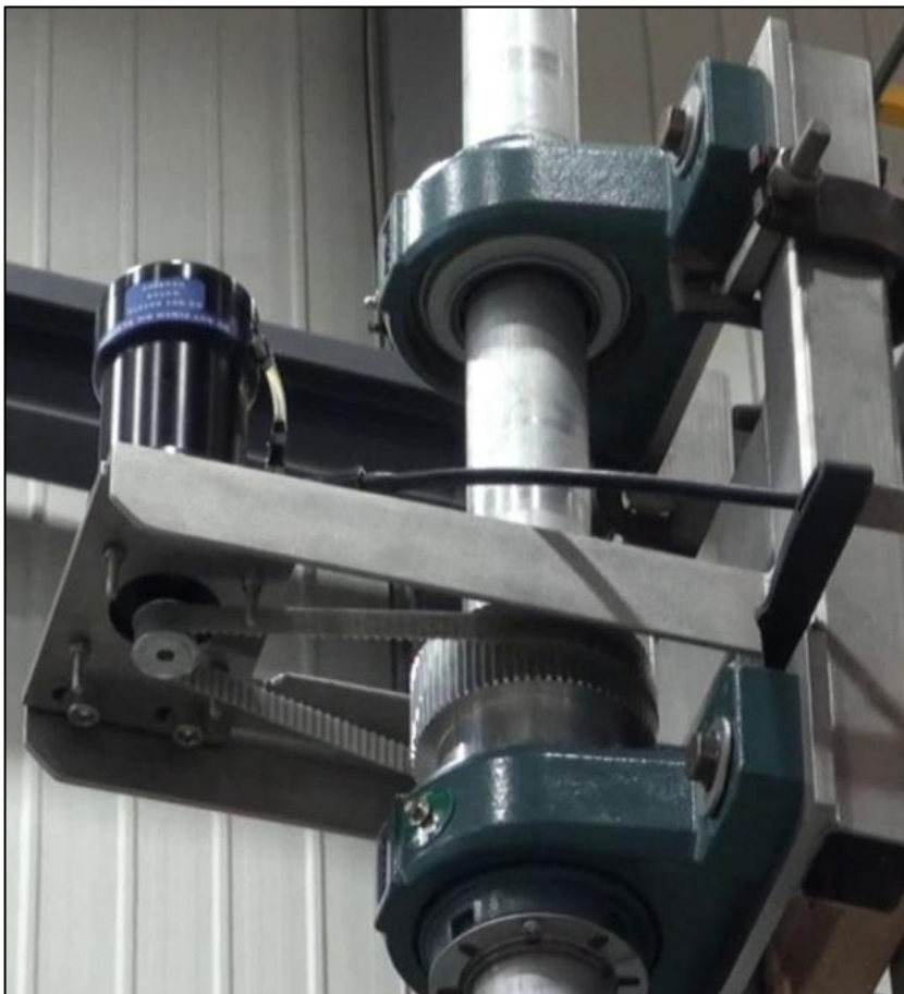
Figure 11 - Surface Controlled Pole Camera Rotation System
