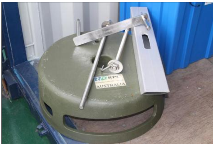
Figure 31 - The "Top Hat" Replacement Hatch Cover
