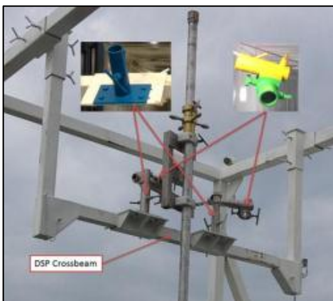
Figure 13 - Dual articulated pole articulation system installed on the DSP crossbeam. (Insets - Colour coded articulation components)
