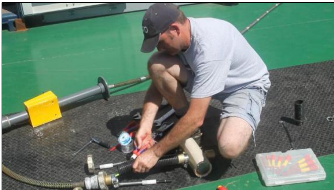
Figure 6 - Illustrating the manner in which the Data Umbilical was fed through to the Camera Module
