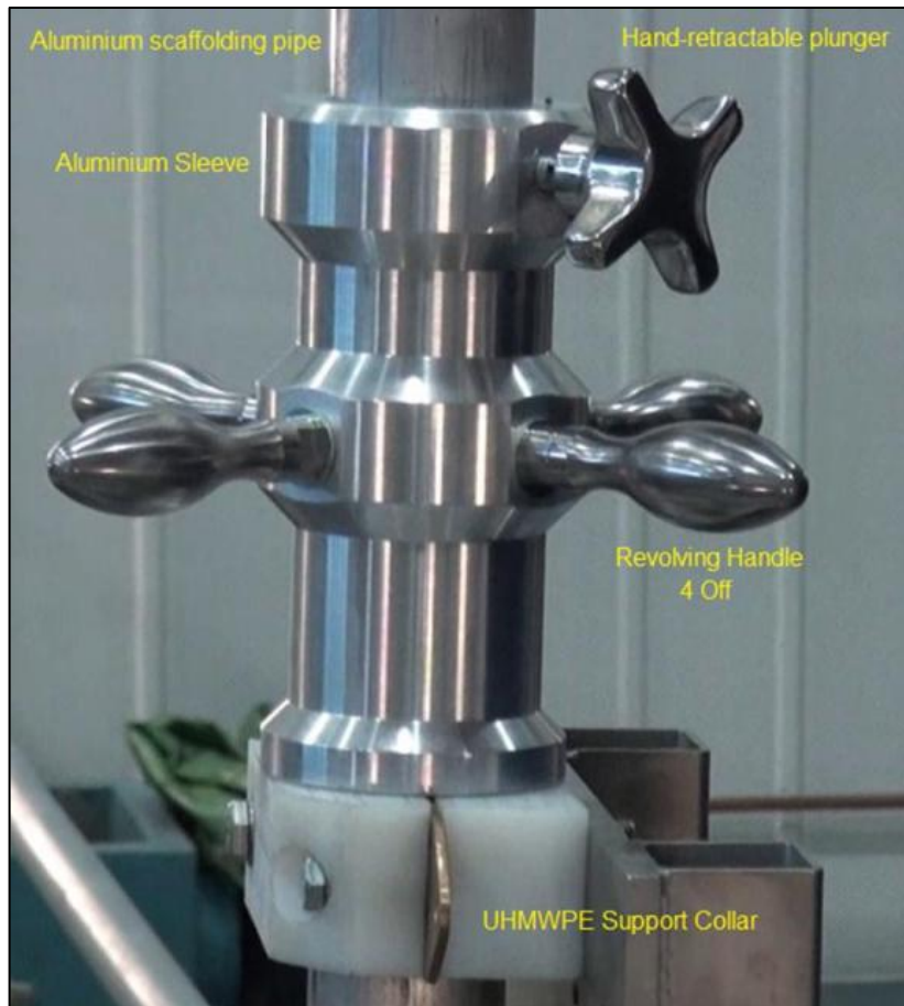
Figure 10 - Diver Operated Pole Cam Rotation System
