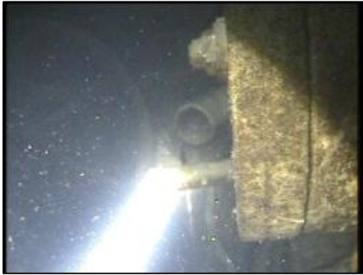
Figure 4 - One of the Lighting Modules showing three of its five LED Arrays
