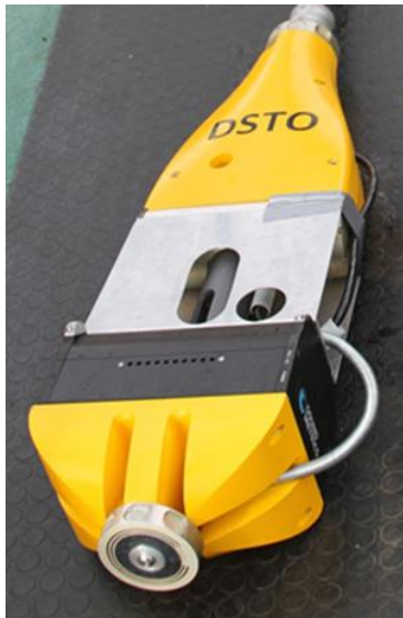
Figure 8 - Two Views of the Instrumentation Pod for the Pole Camera System
