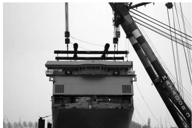
Erecting the superstructure in Rotterdam on 12 February (Photo www.bendijkstra.nl )
