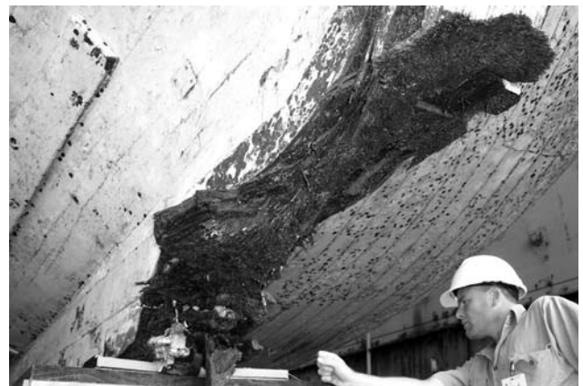
Keel damage showing the protruding rock (Photo courtesy ADI)
