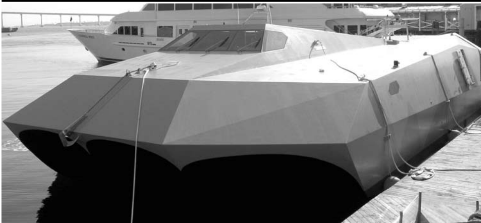
The experimental boat Stiletto is more than 24 m in length and has a carbon-composite hull, which help the boat to travel at speeds more than 50 knots. The boat will be used to transport special operations forces to their mission quickly (US Dept. of Defence photo)
