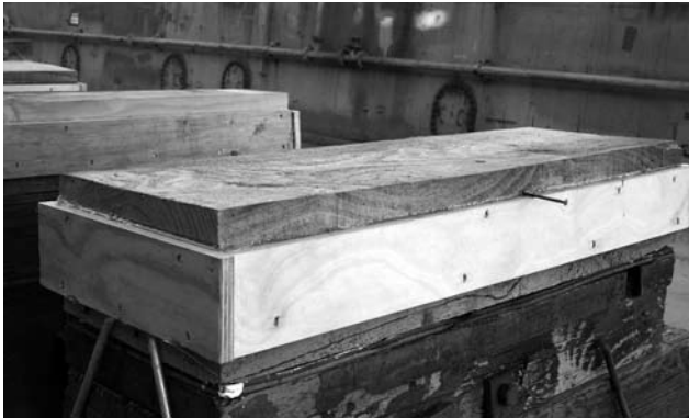
The sand boxes fitted to the keel blocks to enable sections of the keel to be exposed for repair (Photo courtesy ADI)
