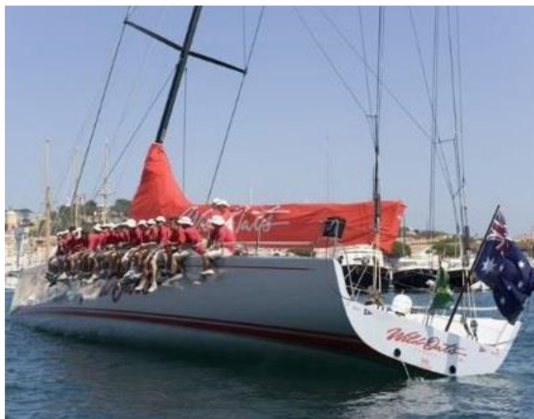
Static load on the windward rail (Photo courtesy Wil Oats Team)
