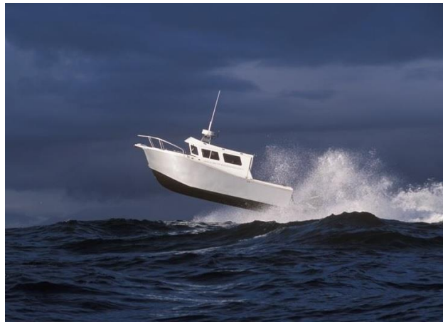
Dynamic load on planing boat (Photo from Noal Boats website)
