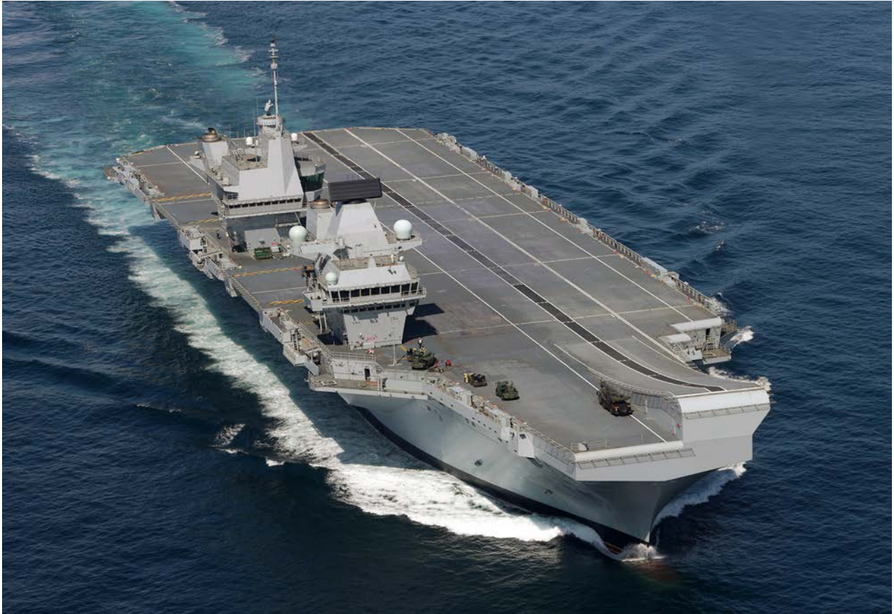
Launched on 17 July 2014, the future HMS Queen Elizabeth left Rosyth Dockyard in Scotland on 26 June 2017 for sea trials. At 70 600 t full load displacement, the 280 m long carrier and her sister ship HMS Prince of Wales are the largest ships ever built for the Royal Navy. Despite her size, the complement of HMS Queen Elizabeth will be a relatively modest 679, made possible by the maximum use of automation throughout the ship (Photo MOD Crown Copyright)
