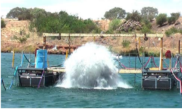
UNDEX trial for measuring the whipping response of a cylinder (Photo courtesy Steven de Candia)
