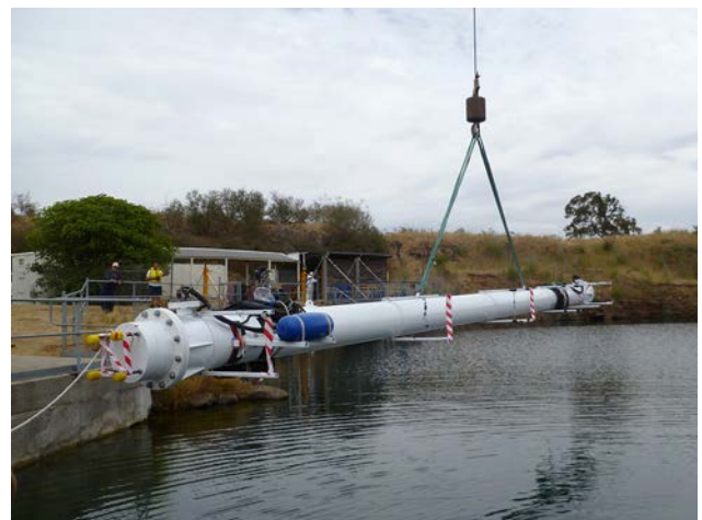
Cylinder for UNDEX trials being lowered into the water (Photo courtesy Steven de Candia)
