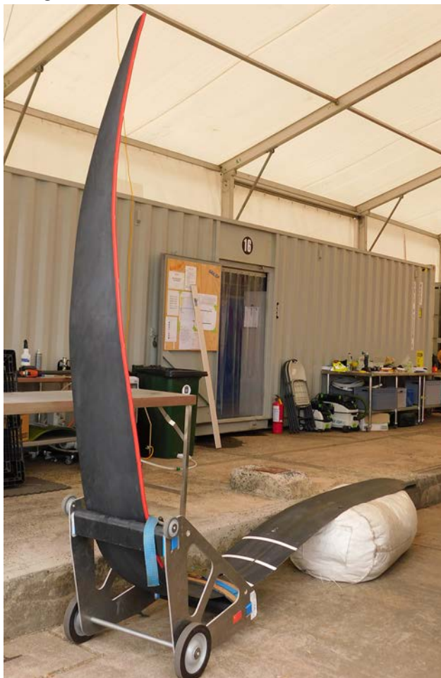
Figure 3: A main foil removed from a boat showing its complex geometry and a temporary protective strip applied to its trailing edge (Photo courtesy Martin Grimm)
