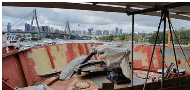
Aft deck with stern bulwarks awaiting fitting of cap rail and steering gear in position (Photo courtesy Andy Munns)
