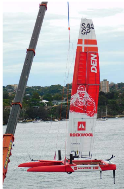
Figure 4: The Danish team boat being lifted from the water showing new wing-sail with flaps and four spanwise segments (Photo courtesy Martin Grimm)
