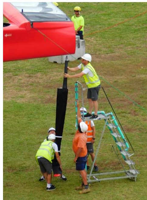
Figure 5: Technical support crew removing a rudder foil to allow the boat to be lowered onto its transport dollies (Photo courtesy Martin Grimm)
