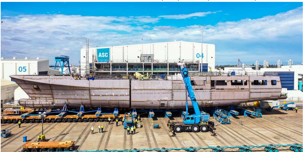
The forward and aft hull modules of NUSHIP Arafura coming together at Osborne recently (Defence photograph)
