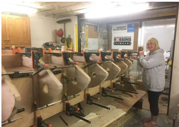
Longbow's sponson frames being installed (Photo from Longbow website)
