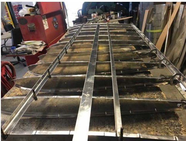
New T-tail for Spirit of Australia 2 under construction (Photo from Longbow website)
