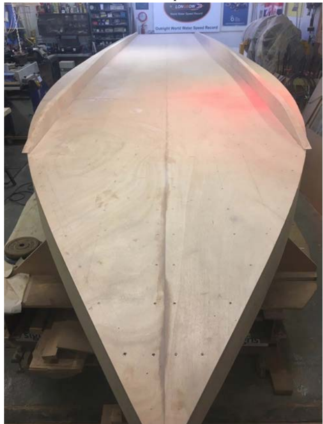
Longbow's side skirts installed completed (Photo from Longbow website)
