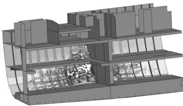
SPH prediction of damage sustained by typical frigate in underwater explosion (Image courtesy Pacific ESI)
