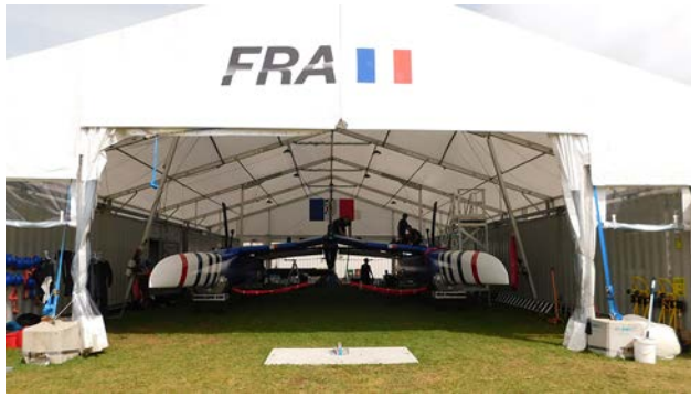
Figure 6: The French team boat stored in the tent hangar constructed in part from the 40-ft containers used to transport the boats between events (Photo courtesy Martin Grimm)
