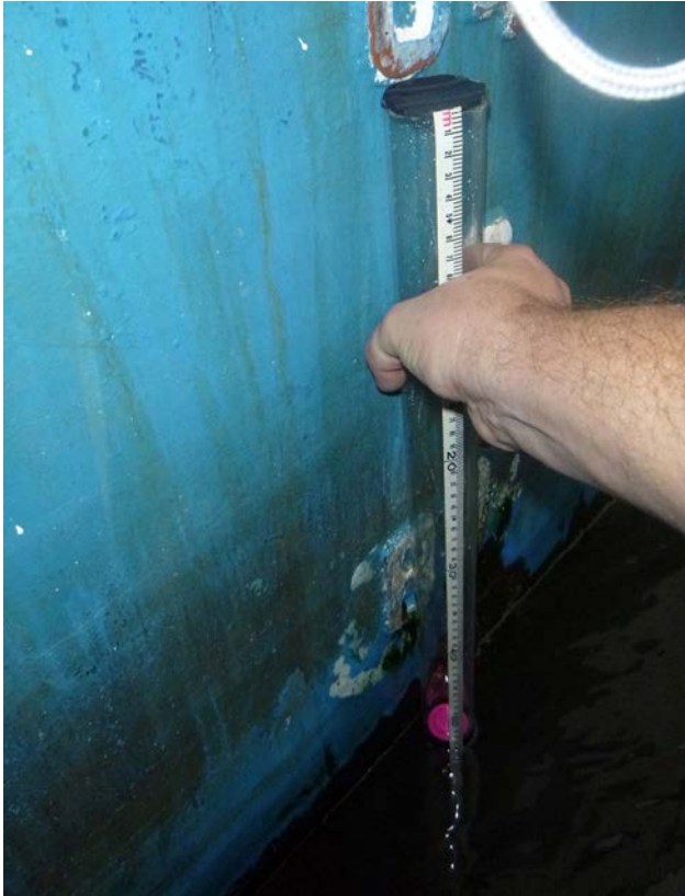
Measuring draft marks on Pacific Explorer (Photo courtesy John Butler Design)
