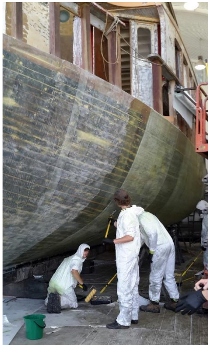
Sheathing Radar's hull with GRP (Photo courtesy Noakes Group)
