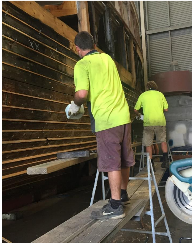
Splining between Radar's planks (Photo courtesy Noakes Group)
