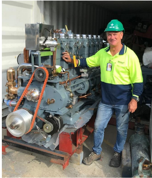
Sean with the overhauled Gardner 8L3B (Photo courtesy Noakes Group)
