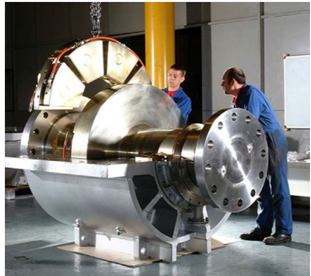
Modern marine thrust bearing (Photo courtesy Michell Bearings)
