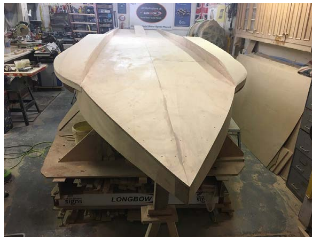
Sponsons and planing shoe complete on Longbow (Photo from Longbow website)
