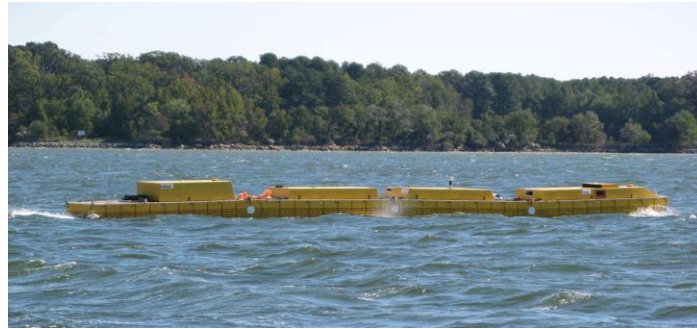
1:20 scale model of the HSS SeaTrain surface-effect-ship being tested on the Severn River near Annapolis, MD, USA (Photo courtesy Alion Science and Technology Corp.)
