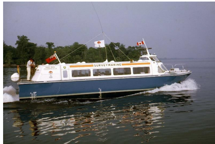
Sidewall hovercraft Hovermarine HM2 Hoverbus in operation (Photo courtesy Lawry Doctors)
