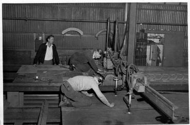
Scrieve boards on which the lines have been adjusted for kerf are fastened to the tracing table of the profile cutter and by means of a manual tracing control, Port and Starboard floor plates are cut to shape simultaneously.
