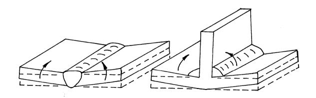
Angular distortion from butt welds is minimised by reducing the eccentricity of the contraction stresses. If the butt weld is completed in one run using a grooved backing bar to support the run on the underside as shown in Fig. 4, there will be relatively uniform heating and shrinkage on opposite sides of the neutral axis of the weld.
