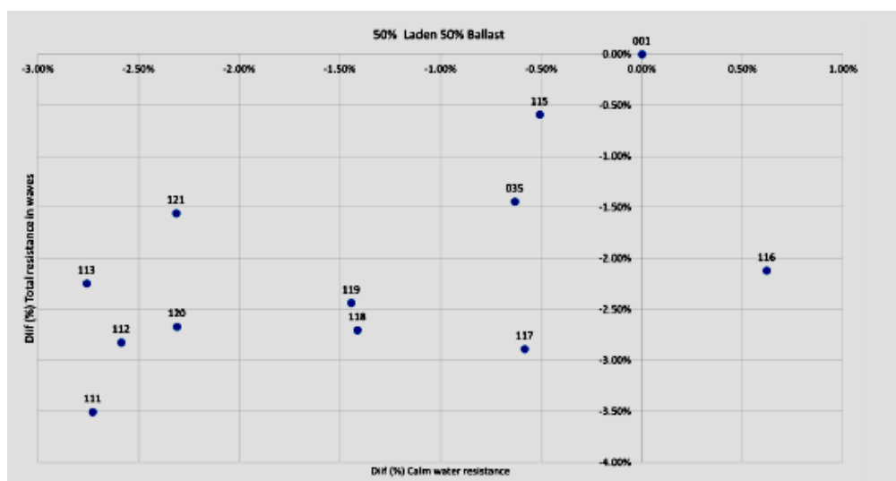
Figure 14: Differences with the initial design regarding the total resistance in waves as a function of the differences with the initial design regarding the calm water resistance.
