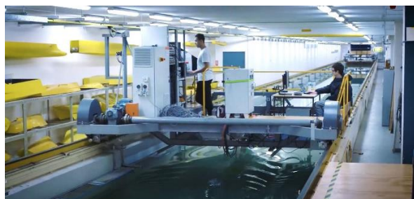
The submarine model being tested in the towing tank (Photo courtesy AMC)
