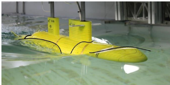
EFD results for model wave generation at 1.12 m/s ( Fr = 0.275 ) (Photo courtesy Mathieu Courdier)
