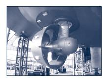
Influenced by IMO regulation on energy efficient design index (EEDI), the demand of energy saving devices (ESDs) is expected to keep growing. Its design requires a deep knowledge of the flow behaviour in the aft area of the vessel and highly advanced CFD simulations are required in order to properly characterise the hydrodynamic efficiency due to the propeller/hull interaction.
