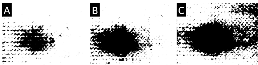
Figure 5: Void Content in Panels filled with full inlet vacuum at pressure (A) 400mbar, (B) 200mbar, (C) 0mbar
