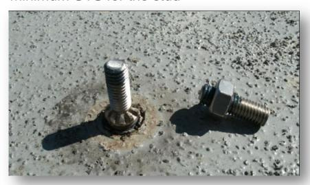
QW-466.5 TORQUE TESTING ARRANGEMENT FOR STUD WELDS
