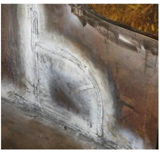
The cracked weld after repair and heat treated
