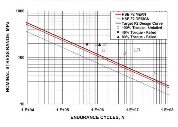
Fatigue test data on subsea 19mm friction stud welds preloaded with a 100% torque of 170 Nm (Series 2 in Ref.3) subject to axial load.
