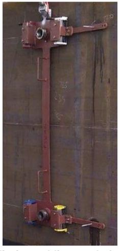
Jig for welding studs for Cofferdam attachment
