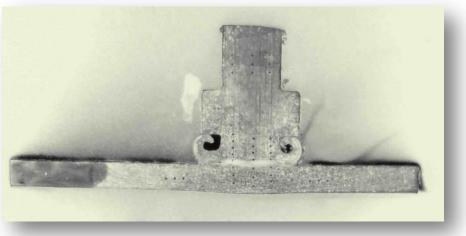
Explosive atmosphere test and macro for M8 friction stud welds on SMO 254 Super Austenitic Stainless Steel. The pipe is 3mm wall thickness and contains a water glycol mixture.
