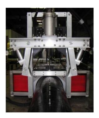
Testing the HMS3000 stud welding system in the ROV tool skid
