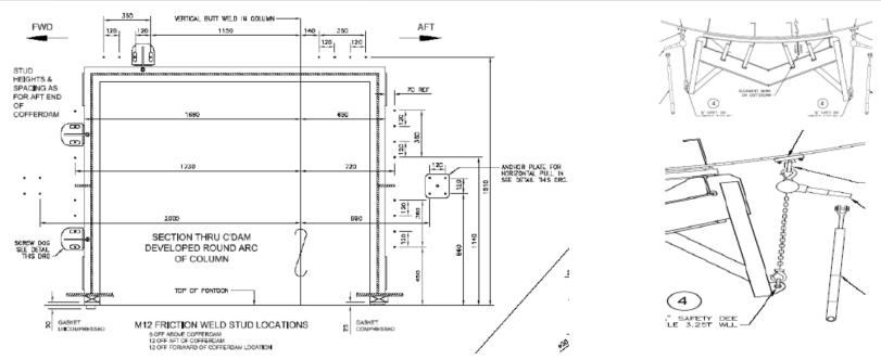
Subsea friction stud weld locations for the cofferdam attachment to the FPS hull
