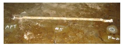
Anodes after 12 years service in an FPSO oil storage tank.
