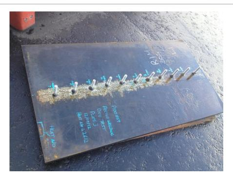
One of three test plates stud welded for fatigue testing by DNV
