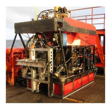
The ROV with the stud welding tool skid
