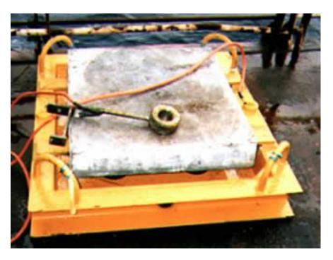
Anode skid with the continuity tail ready for Tri-partite friction stud welding
