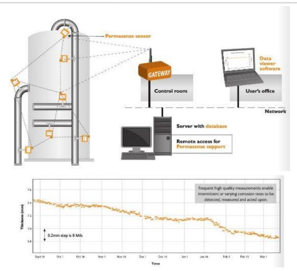
Continuous corrosion monitoring using wireless waveguide based ultrasonic thickness measuring sensors.
