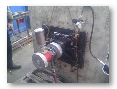
Proserv's R1400 pneumatic tool was used for retrofitting 160 anodes in a oil storage tank on the Terra Nova FPSO in Zone 1.
