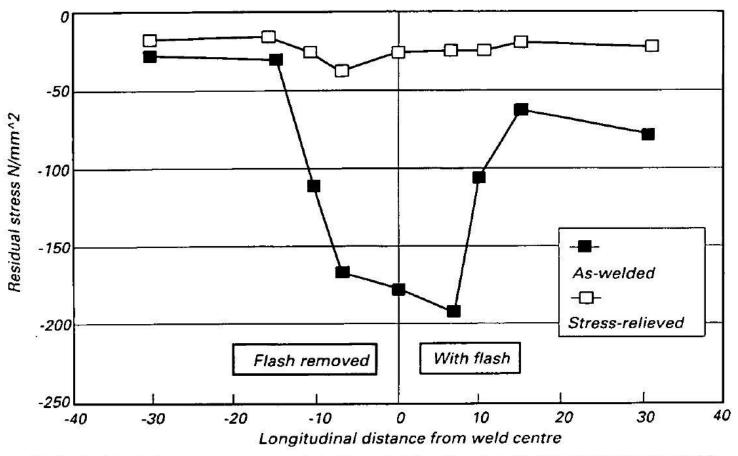
Fig.5 Residual stress measurements in the axial direction (i.e. perpendicular to the weld) obtained from specimens 77210-23 and 77210-24 representing the stress relieved and as-welded conditions, respectively.
