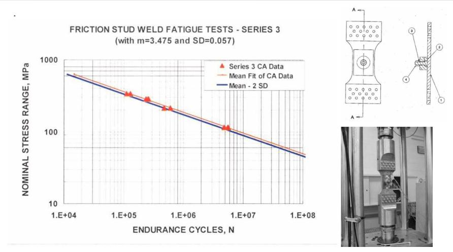
C1 Curve from underwater fruiction stud welds. Fatigue tests representing the presence of a friction weld on the moon pool hull plate as it sustains global bending without the live load applied through the stud
