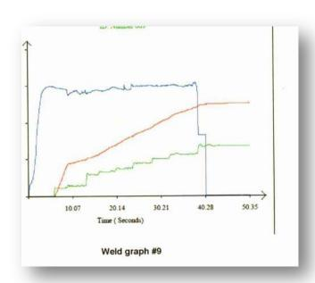
Typical data from the friction welding control system: Rotational speed, ram pressure and "Burnoff". The tool can also perform a tensile test if required.
