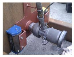
R1004 Friction welding tool in a magnet clamp
