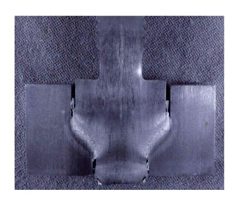
Friction plug weld on 40mm thick S32760 Super Duplex Stainless Steel
