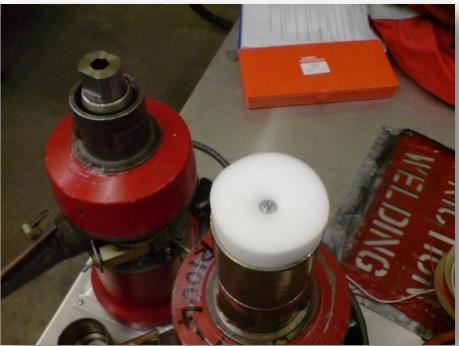
The stud weld is encased within a foam and metal shroud. In addition, for welding in zoned areas a water spray can also be applied during the welding and spark arrestors are fitted to the air exhaust.
