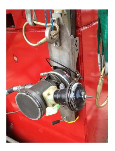
A stud for attaching a fire wall friction welded to the accommodation module on the platform
