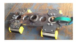
A jig for locating the friction stud welding tool
