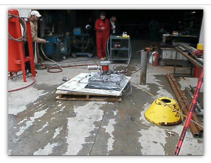
After the weld has been completed the gas mixture of 14% Acetylene and air is detonated to verify that the gas was explosive.
