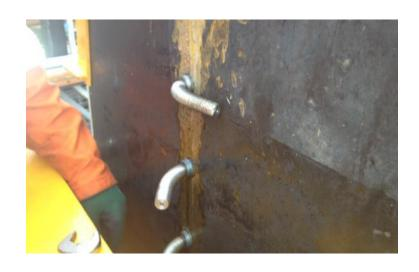
Bend tests on M16 underwater stud welds
