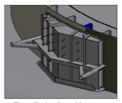
The cofferdam in position over a crack in a weld between a column and a pontoon on an FPS
