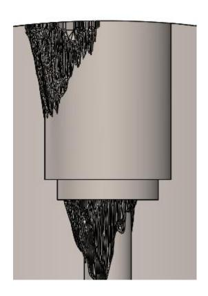
Hole eroded by cavitation machined for friction plug weld
