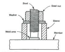
(a) Dimensions are appropriate to the size of the stud. (b) Threads of the stud shall be clean and free of lubricant
