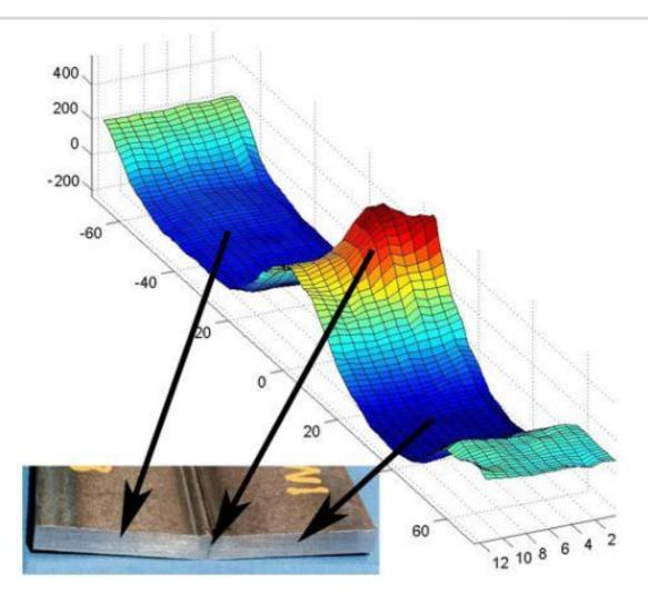
Typical residual stress pattern for a fusion butt weld made with arc welding
