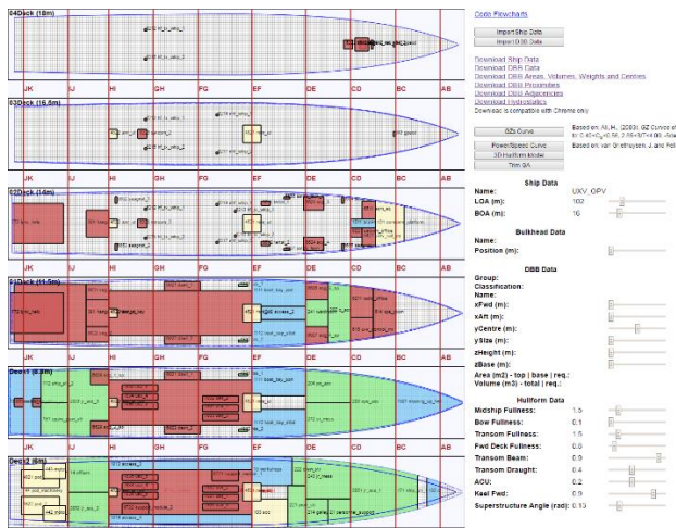
Figure 28: Deck Plans of a typical ESSD model in the UCL Layout tool (Pawling et al, 2015)
