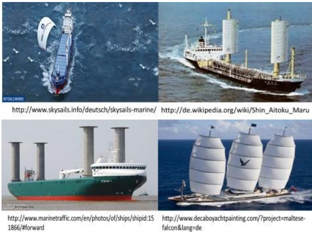
Figure 1: Different wind propulsion systems (WPS) used for wind assisted ship propulsion (WASP): a kite (top-left), Flettner rotors (bottom-left), soft furling square sails (Dynarig sails on the Maltese Falcon, bottom-right), solid foldable square sails with a similar function as the Dynarig (Shin Aitoku Maru, top-right).
