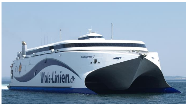
Figure 1. A photo of Mols-Linjen 112 m wave piercing catamaran with centre bow built by INCAT Tasmania ( www.INCAT.com.au , 2017)
