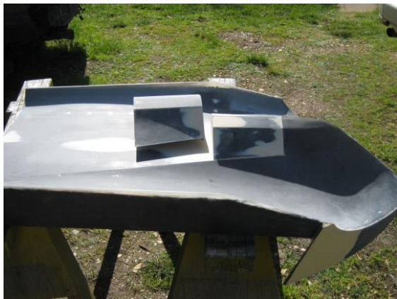
Figure 9: Three centre bow length segments of HSM02 under construction. The short centre bow was achieved by cutting 150 mm from centre bow aft end and a separate segment was built to form the long centre bow.
