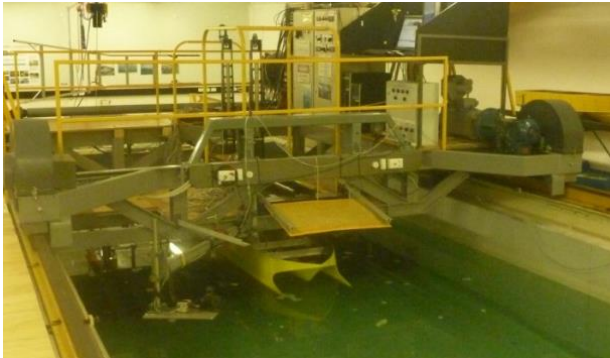
Figure 10: The AMC towing tank carriage and the HSM02 in the water
