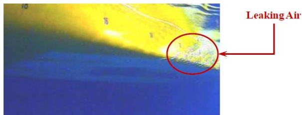
Figure 20 Captured air layer at VS = 14.5knots (Yoshiaki, et al, 2000)
