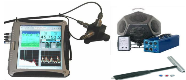
Figure 9: Instrumentation for N&V measurements on board
