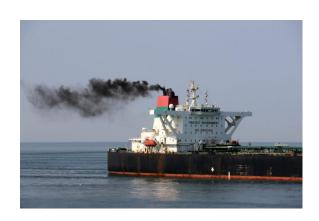
Over several years the IMO have regulated on a reduction in ship engine exhaust emissions of sulphur oxide from the burning of high sulphur fuels. As of the first of January 2020 the maximum fuel sulphur level permitted on a global basis will be a maximum of 0.5% down from the 2019 level of a maximum of 3.5 %. Ship owners and shipping organisations have Expressed concerns on how these changes can be safely and efficiently met.
