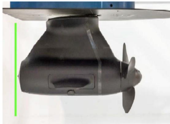
MARIN's pod model with forward propeller, and the green line showing the measurement plane of the PIV system to determine the wakefield flow into the aft propeller (Photo from MARIN Report 27507-6-DT, courtesy Defence)
