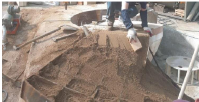
Setting up the mould for one of the new propellers (Photo courtesy Defence)
