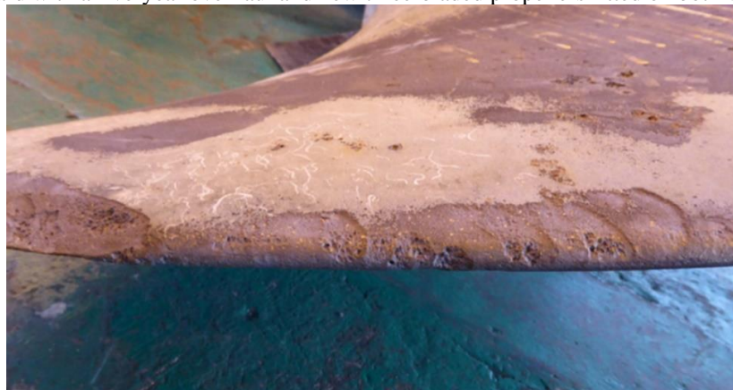
HMAS Adelaide propeller blade with tip-vortex cavitation and corrosion material removed at May 2017 dry docking after 19 months in service (Photo courtesy Defence)
