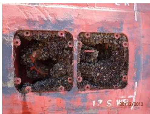
Fouling on a tug in Cockburn Sound, WA (Photo courtesy John Lewis)
