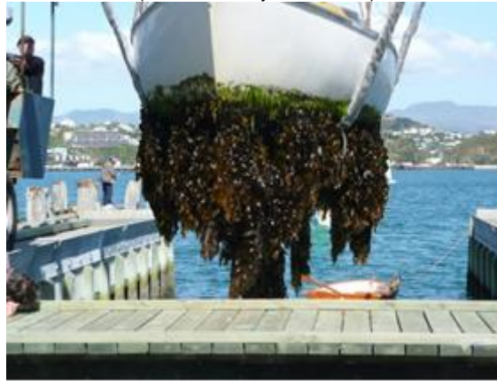
Fouling on a yacht left too long in the water! (Photo courtesy John Lewis)
