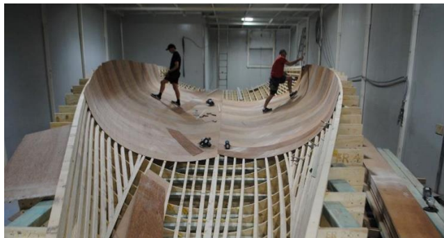
Plywood being installed (Photo courtesy McConaghy Boats)
