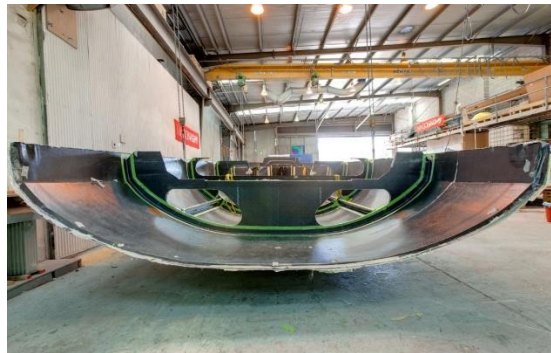
Installation of bulkheads (Photo courtesy McConaghy Boats)
