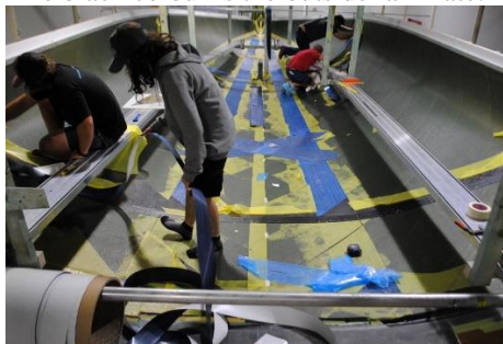
Laminating the hull outside skin (Photo courtesy McConaghy Boats)
