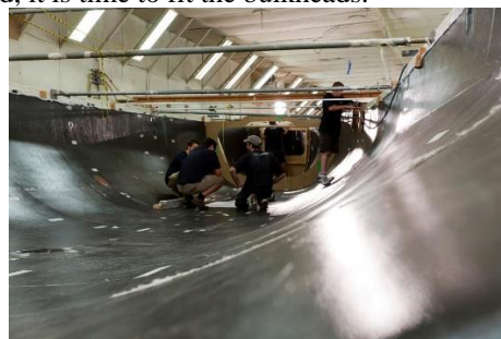
Hull shell completed (Photo courtesy McConaghy Boats)
