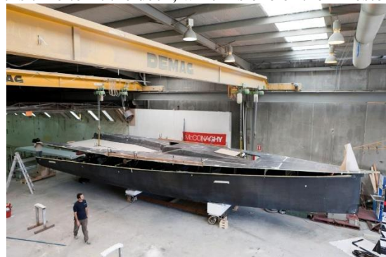
Fitting the deck (Photo courtesy McConaghy Boats)
