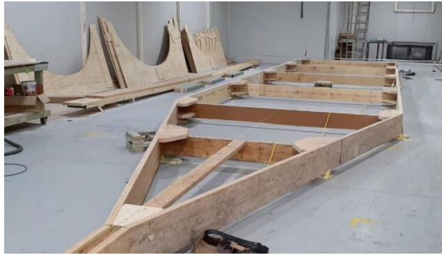
Base jig, centreline string and frames stacked at side (Photo courtesy McConaghy Boats)
