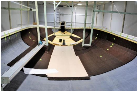
Fitting the honeycomb core (Photo courtesy McConaghy Boats)
