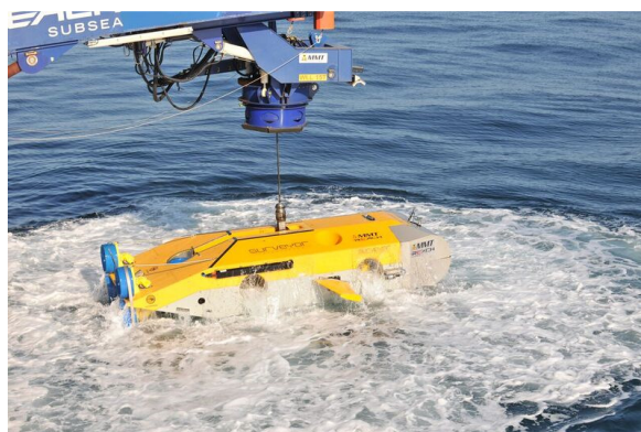
Image: Farr 2016 Launching the ROV Surveyor Interceptor (Reach Subsea, MMT, EEFE)
