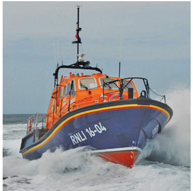
RNLI Tamar class lifeboat - FRP construction
