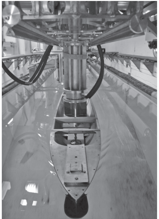
A modern towing tank.
