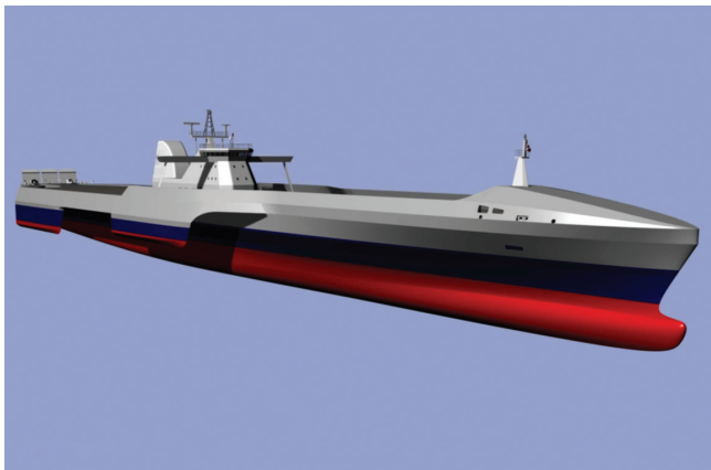
240m 40kt Pentamarin RoRo - a concept by BMT Nigel Gee Ltd.
