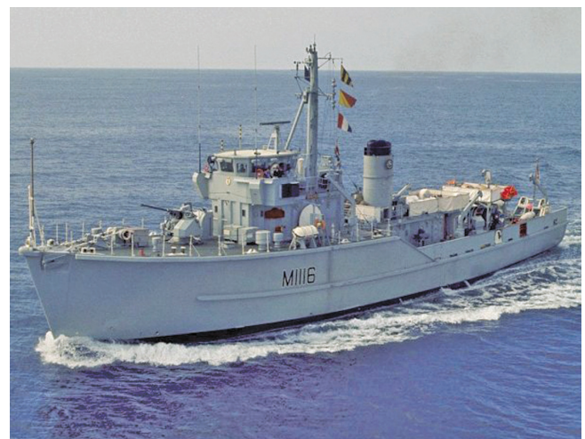
HMS Wilton was the first warship in the world to be constructed from glass reinforced plastic
