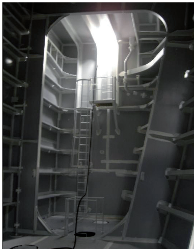
Ballast tank – showing complexity of structure that has to be coated
