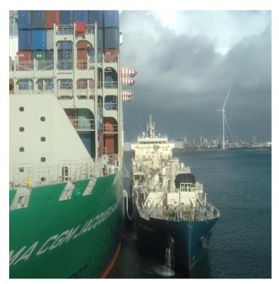
As the world strives towards reducing the effect of global heating it has been identified that emissions from ships need to be cleaned up and so the search for alternative fuels began. LNG has almost always been used as a fuel for LNG ships that carry LNG as a cargo as this was the principal way in which the boil off gas generated by an LNG cargo was controlled.
