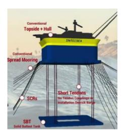
The novel LM-FPSO design is a result of several-year technology development which undergone extensive model tests, reviews at open industry meetings, and received Approval in Principle from DNV. This presentation will discuss the key components of the system and its differentiators, will show its motion performance by predictions and model tests, and will explain the construction and installation sequence.
