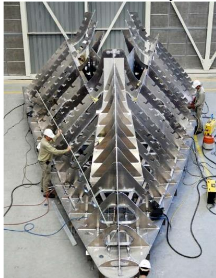
Bow module under construction (Photo courtesy SilverYachts)
