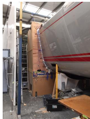
Hull join being vacuum bagged
