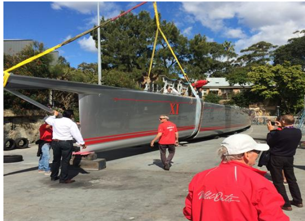
Wild Oats XI with the 11.2 m bow section cut away (Photo courtesy Diab Group)
