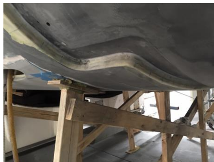
Hull ready for joining (Photo courtesy Diab Group)
