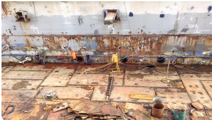
Doubler plates on the pontoon deck (Photo courtesy Noakes Group)
