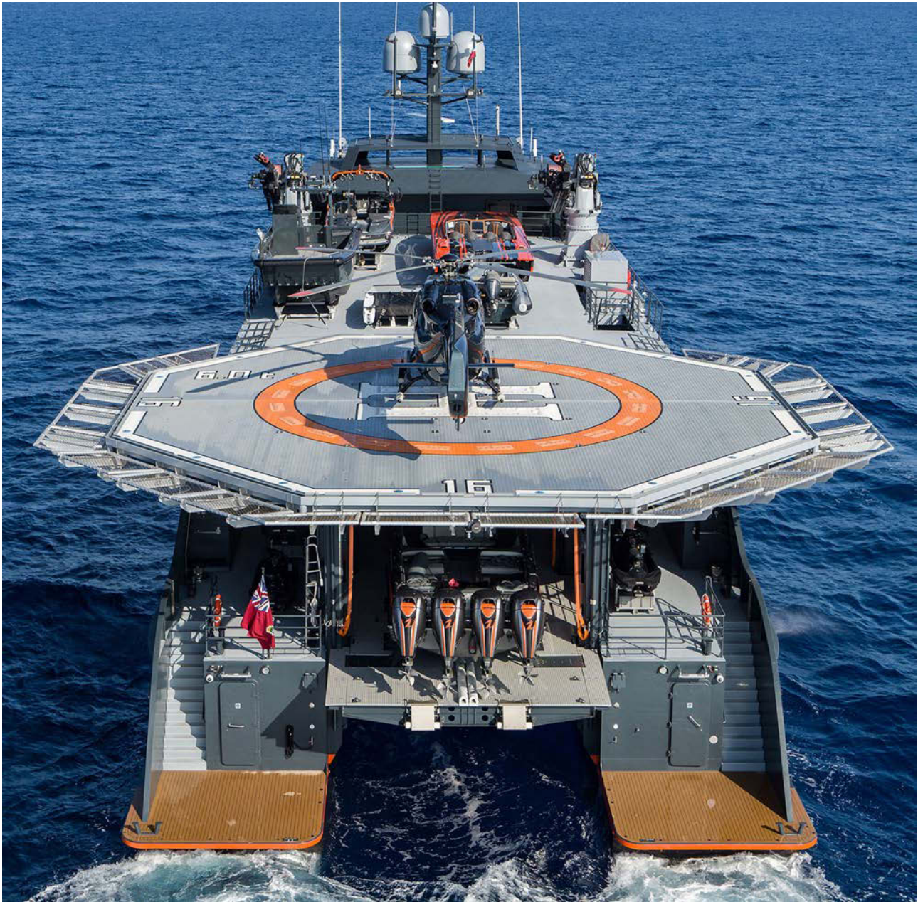
Bristling with toys, the shadow cat Hodor was designed by Incat Crowther and built by Astilleros Armón at their Burela shipyard in Spain. The 66.2 m catamaran can carry five tenders (from 7 m to 17 m in length), four jet skis, four quad bikes, an Aurora-5 submarine with its own garage, a helipad, and a large complement of crew, staff and support equipment (Photo courtesy Incat Crowther)
