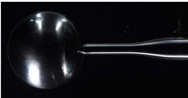
Sphere setup within the cavitation tunnel (Photo courtesy Australian Maritime College)
