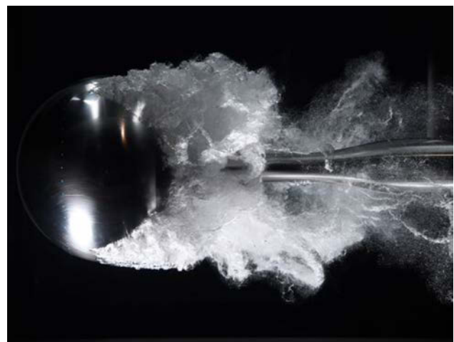
The development of cavitation at \sigma = 0.59 and Rn = 3 \times 10^6 for the stainless steel sphere (Photo courtesy Australian Maritime College)
