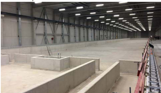
The new shallow-water towing tank in Ostend, with composite tank floor, carriage and wave-maker to come (Photo courtesy Tim Gourlay)
