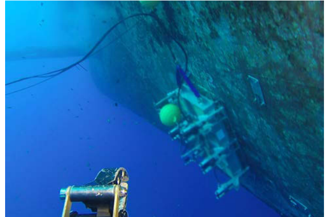
Diverless sea-chest blanking (Photo courtesy Stuart Barrow)
