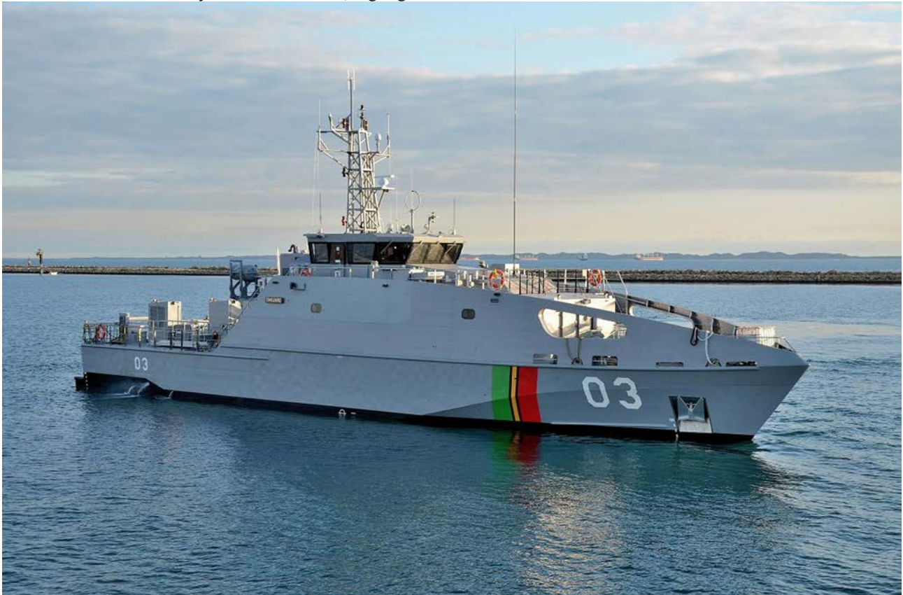
Vanuatu's RVS Takuare is a 39.5 m steel monohull Guardian-class patrol boat designed and constructed by Austal in Henderson, Western Australia (Photo courtesy Austal)
