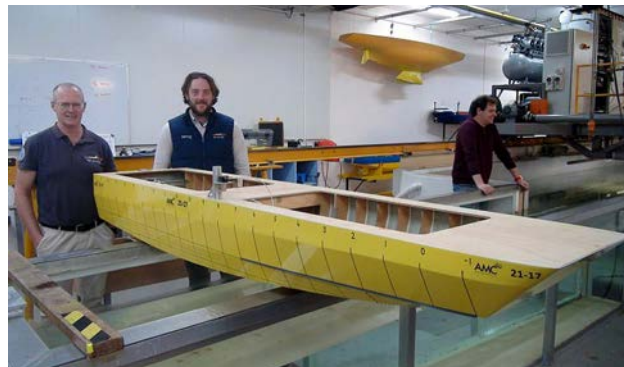
The model of Oboe 1 at the AMC test tank (Photo courtesy AMC)
