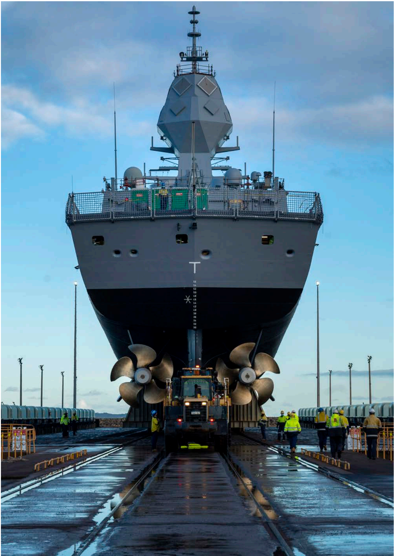
HMAS Perth is moved onto the ship lift at the Australian Marine Complex at Henderson, WA, for undocking after completing a major part of the Anzac Midlife Capability Assurance Program to upgrade radar and communications systems and crew habitability (RAN photograph)
