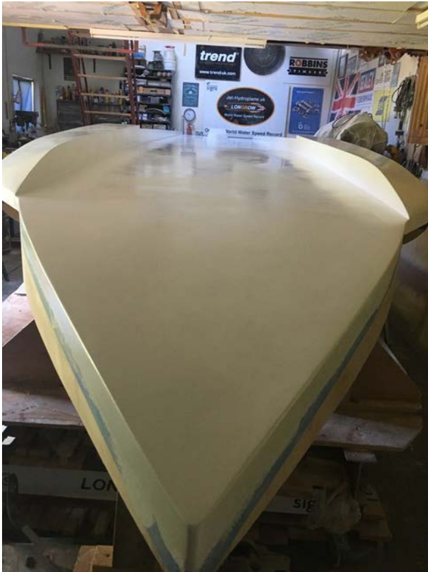
Longbow's underside coated with HMG primer (Photo from Longbow website)
