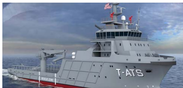
Austal USA will prepare a functional design for the new Navajo-class Towing, Salvage and Rescue Ship (T-ATS) for the US Navy, an 80 m steel monohull with multi-mission capability to support a variety of towing, salvage, search-and-rescue, oil-spill response, humanitarian assistance and surveillance activities (Image courtesy Austal)
