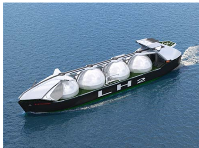
An impression of a large liquefied hydrogen carrier with a cargo carrying capacity of 40 000 m 3 per tank in four tanks (Image courtesy of Kawasaki)
