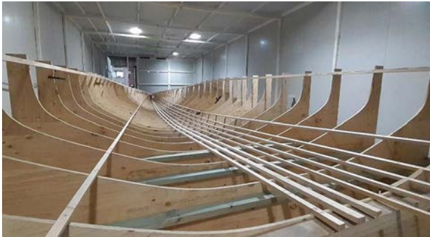
Frames up and stringers going in (Photo courtesy McConaghy Boats)
