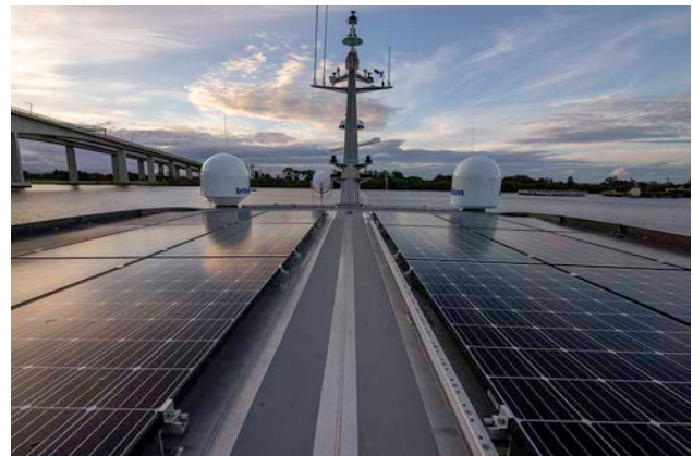
Solar panels on the upper deck of Reef Resilience (Photo courtesy Incat Crowther)
