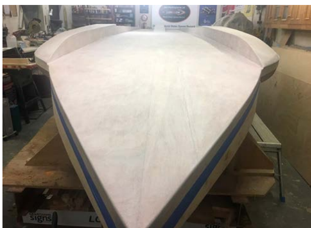
Longbow's underside sheathed in Dynel and epoxy resin (Photo from Longbow website)
