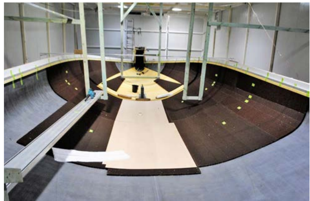
Fitting the honeycomb core (Photo courtesy McConaghy Boats)
