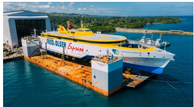
Austal Philippines launching Bañaderos Express using their recently-acquired floating dock (Photo courtesy Austal Philippines).
