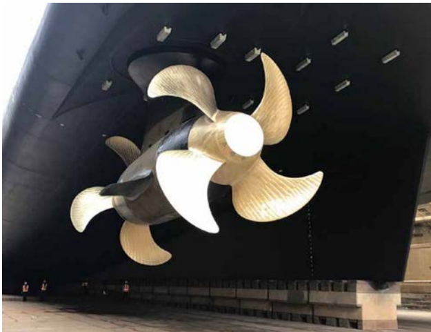
Ready for undocking — HMAS Canberra 's new pods have four bladed propellers. The ship's original propellers had three blades (RAN Photograph)
