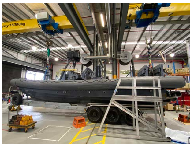
Inclining of 11 m RHIB in air (Photo courtesy John Butler Design)
