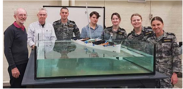
In the lab for the model inclining experiment at UNSW Canberra (Photo courtesy Warren Smith)
