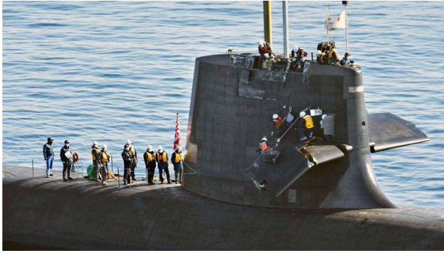
Damaged fin on sail of Japanese submarine Souryu (Photo from BBC website)
