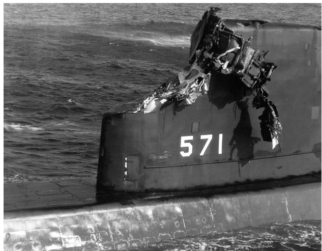
Damaged sail on USS Nautilus (SSN 571) (Photo from NavSource website)
