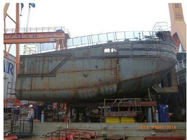
Bow section block under construction (Photo courtesy Neil Edwards)
