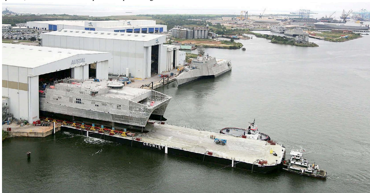
Trenton (JVSV 5) emerging from Assembly Bay 3 at Austal USA's shipyard (Photo courtesy Austal)
