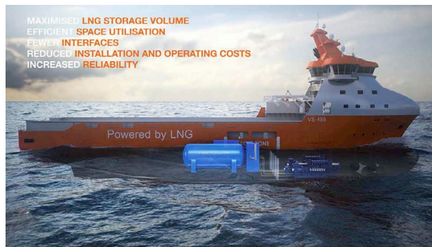
The Wärtsilä LNGPac system installed in a platform supply vessel (Image courtesy Wärtsilä)
