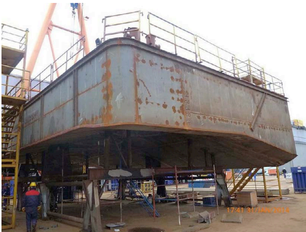
Aft section block under construction (Photo courtesy Neil Edwards)
