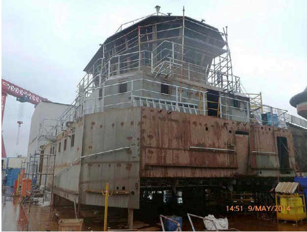
Wheelhouse block under construction (Photo courtesy Neil Edwards)
