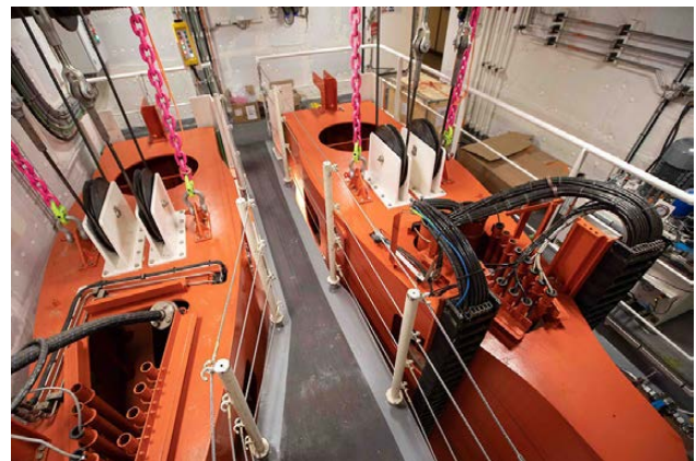
Two 'drop keels' with acoustic instruments can be lowered below the ship's hull to avoid interference from ice or bubbles (Photo Pete Harmsen courtesy AAD)
