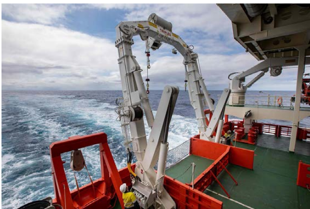
The A-frame for deploying nets and other equipment from the trawl deck (Photo Pete Harmsen courtesy AAD)
