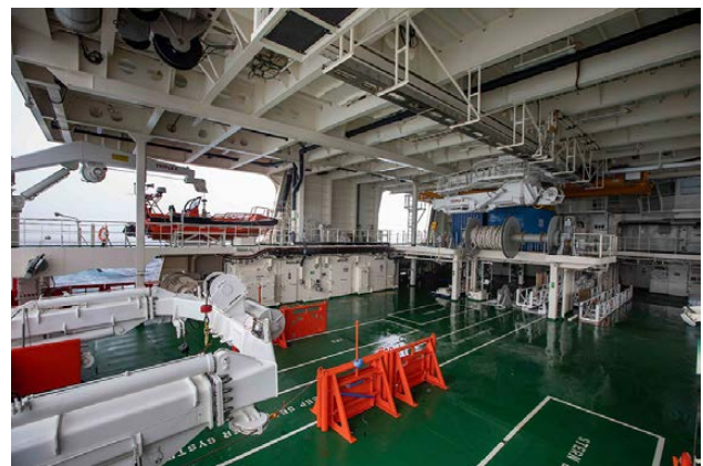
The trawl deck showing A-frame, winch systems, net drums, cranes and one of the personnel tenders (Photo Pete Harmsen courtesy AAD)
