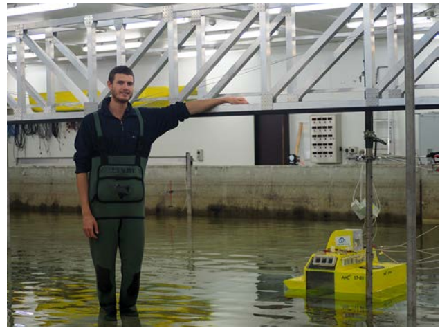
PhD candidate Jarrah Orphin conducts tests on a model wave energy converter in the model test basin at the Australian Maritime College (Photo courtesy AMC)
