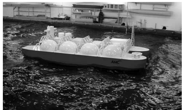
The GasCat, a novel LNG floating production and storage facility being investigated in the AMC Model Test Basin for a collaborative project with Woodside and WA Energy Research Alliance in 2008 (Photo courtesy AMC)
