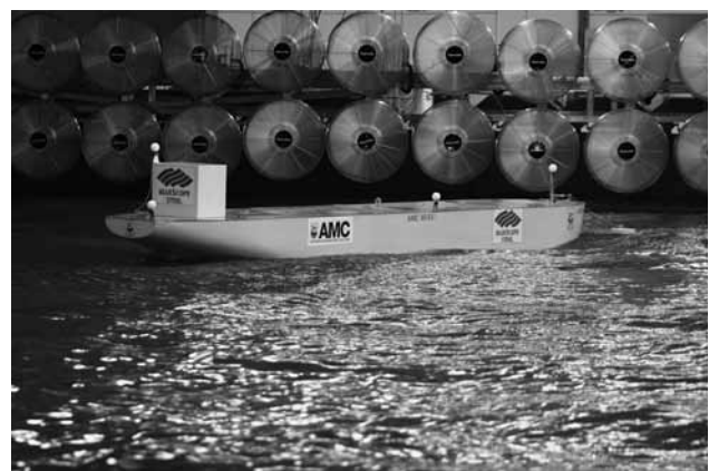
A 4.2 m long scale model of a bulk carrier experiencing both wind and waves within the AMC Model Test Basin in 2007 (Photo courtesy AMC)
