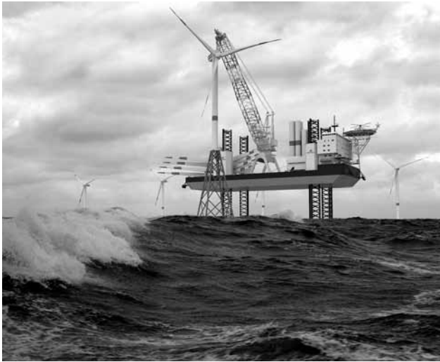
The Turbine Installation Vessel can operate in year-round weather conditions with an operational water depth range of 4.5 to 50 m (Image courtesy Wärtsilä)
