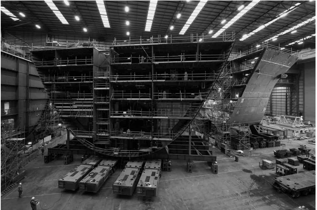
Modules for the first of the Royal Navy's new aircraft carriers, Queen Elizabeth , continue to take shape in yards in the UK. This photograph shows a ring being moved into position for consolidation into a major module at Portsmouth in February. The operation appears to be largely under the control of the man in the bottom left of the photograph (Photo courtesy BAE Systems)
