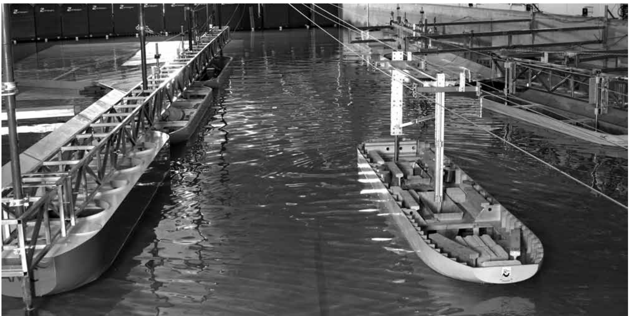
A physical model of a shipping port. These experiments will quantify the hydrodynamic effect of a ship (centre foreground) as it passes several berthed vessels at a known speed. In such scenarios the bathymetry of the shipping channel is also accurately modeled (Photo courtesy AMC)
