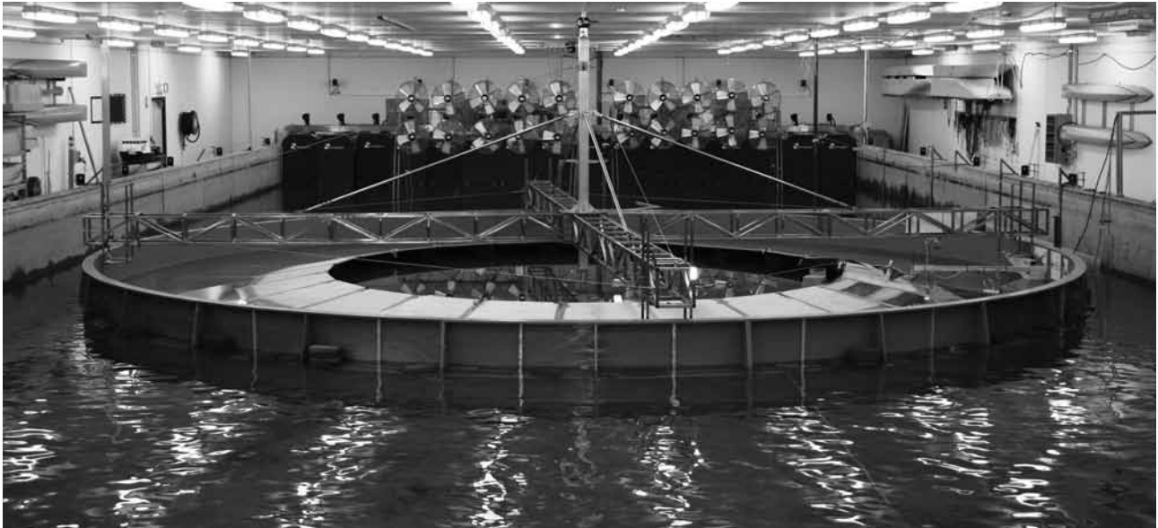
A 10 m diameter scale model of the Webber Wave Pool, including rotating arm, set up in the AMC Model Test Basin in 2010 (Photo courtesy AMC)
