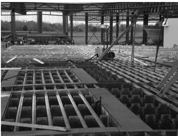
Main deck structure of 58m catamaran crew Boat under construction at Gulf Craft (Image courtesy Incat Crowther)
