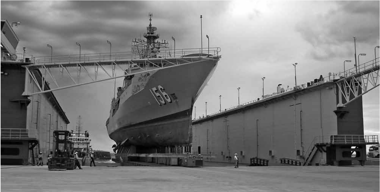
HMAS Toowoomba in the floating dock with the SPMTs in position (Photo Hugh Hyland)
