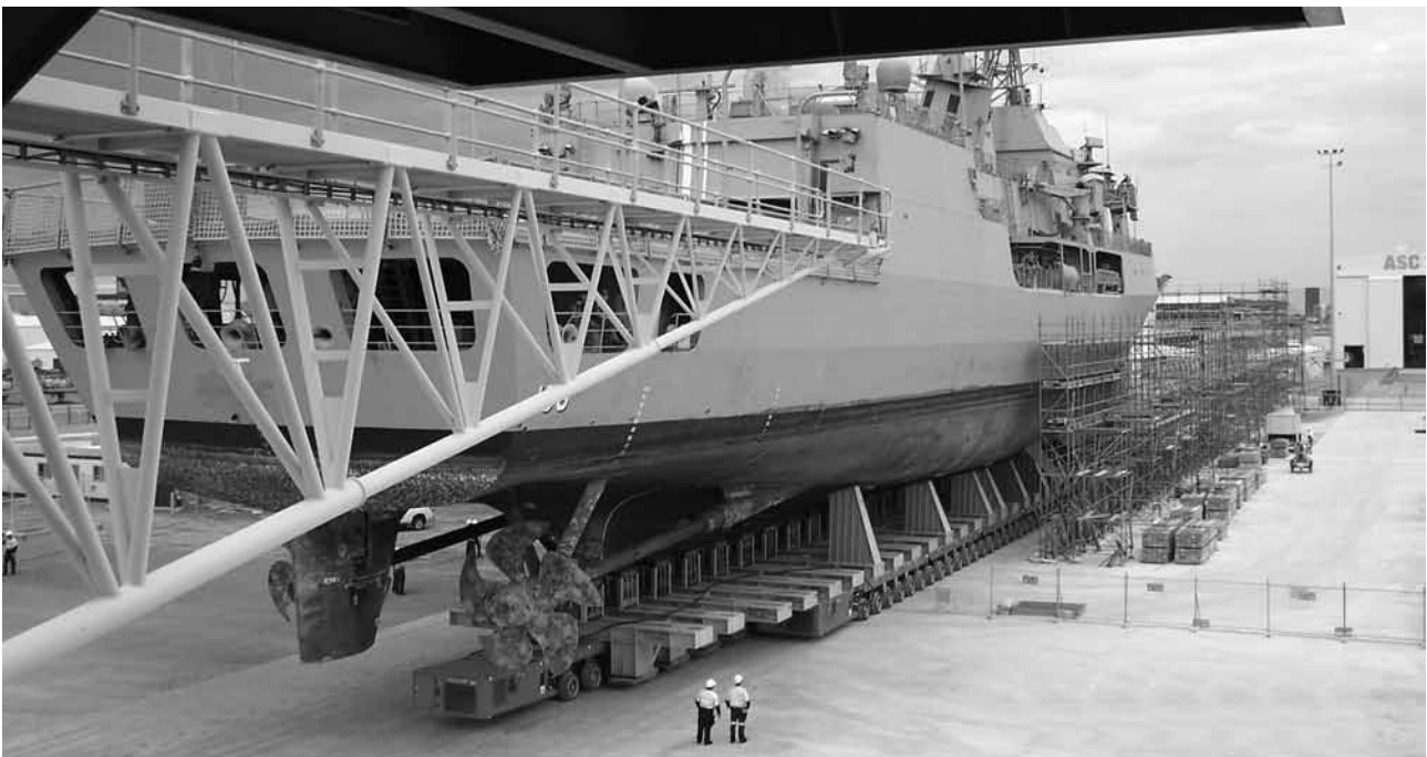
HMAS Toowoomba ashore. Note how the docking cradle is supported by the SPMTs. The submarine HMAS Waller is in the ASC facility in the background and HMAS Farncomb was nearby at the adjacent BAE Systems shiplift (Photo Hugh Hyland)
