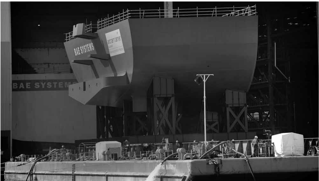
Lower Block 05 of HMS Queen Elizabeth being prepared for transport to Rosyth from Portsmouth in April (Photo courtesy BAE Systems)
