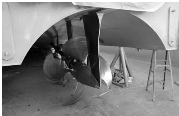
New controllable-pitch propeller and rudder on Seastreak Wall Street (Photo courtesy Incat Crowther)
