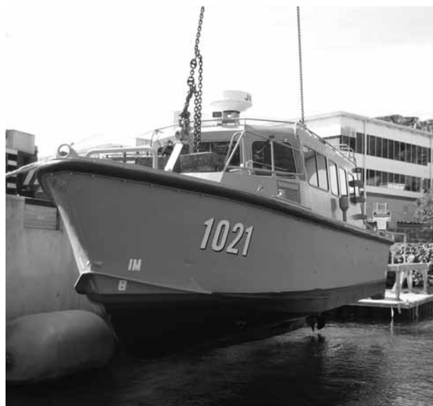
Lifting of SMB Conder prior to inclining (Photo courtesy BCTQ)
