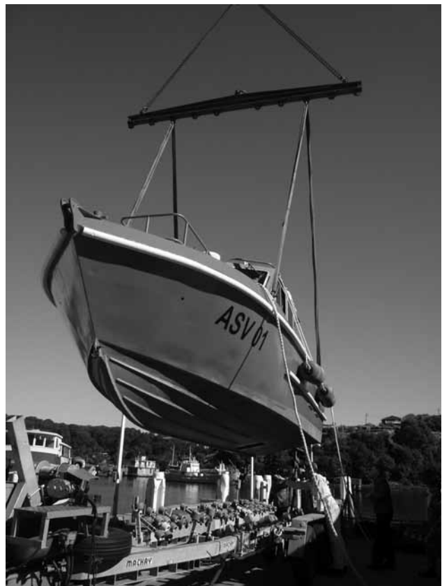
Lifting of ASV Wyatt Earp prior to inclining (Photo courtesy BCTQ)
