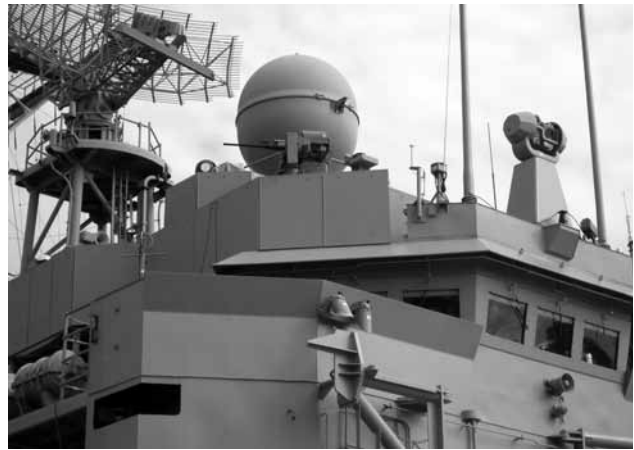
Ballistic panels on HMAS Melbourne (Photo courtesy BCTQ)
