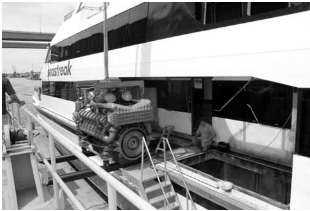
New MTU engine being fitted to Seastreak Wall Street (Photo courtesy Incat Crowther)
