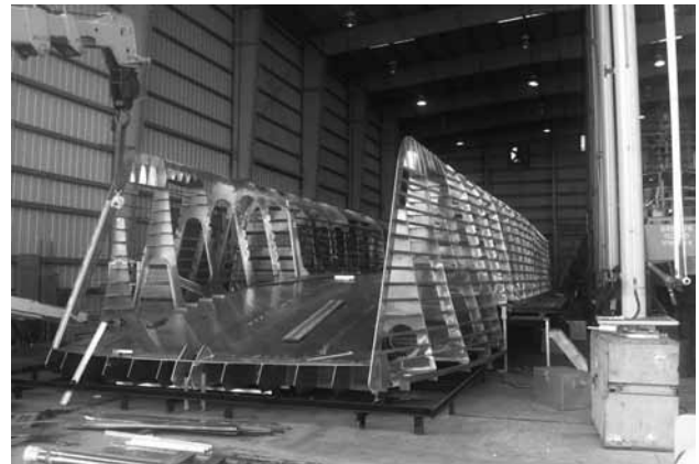
First of the 25 m catamaran passenger ferries under construction at Midship Marine (Photo courtesy Incat Crowther)
