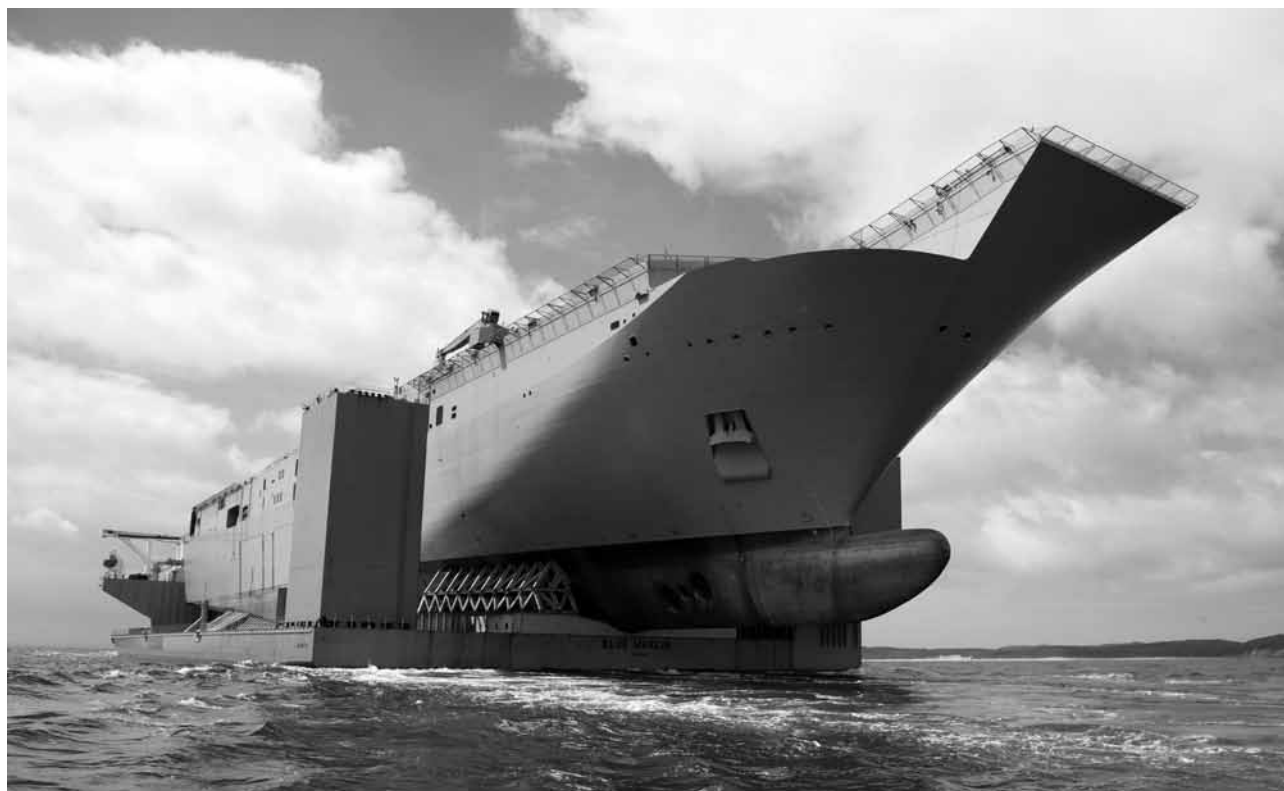
The RAN’s first LHD, Canberra , arrived in Port Phillip Bay on 17 October on board the heavy lift ship Blue Marlin . Canberra is now alongside at Williamstown where BAE Systems will fit the superstructure and complete fitting out and trials. HMAS Canberra will join the fleet in 2014 and her recently launched sister ship, the future HMAS Adelaide , will be commissioned in 2016. (RAN Photograph)
