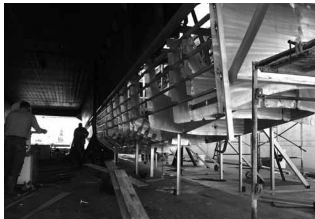
Re-construction work on the underside of the aft end of the starboard hull on Seastreak Wall Street (Photo courtesy Incat Crowther)
