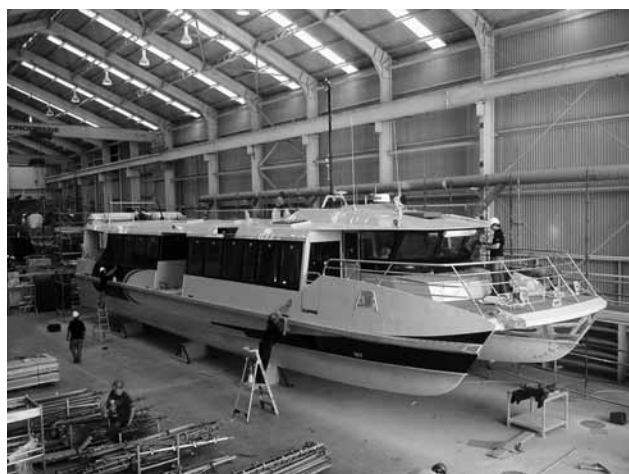
24 m eco-ferry for Nigeria under construction at Aluminium Boats Australia (Photo courtesy One2three Naval Architects)
