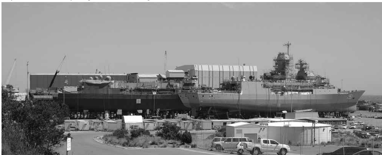
HMA Ships Anzac and Arunta undergoing major refits at the BAE Systems facility in WA. The work includes the fitting of the CEAFAFAR phased-array radar (Photo John Jeremy)
