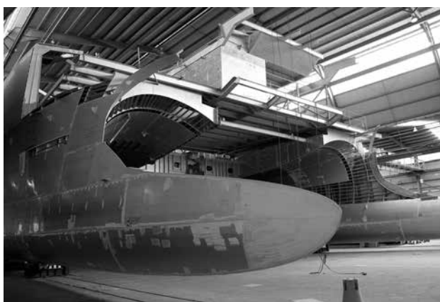
Incat Hull 068 under construction (Photo courtesy Incat Tasmania)
