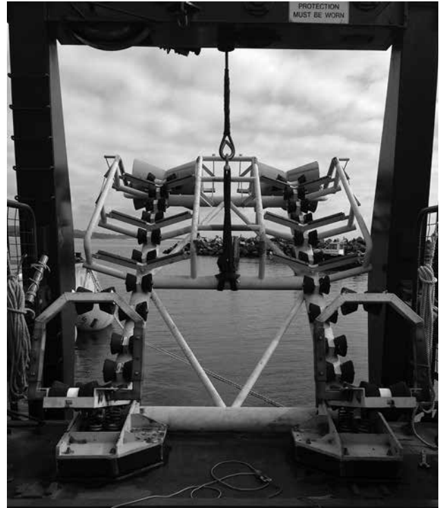
Torpedo recovery system installed on Seahorse Horizon (Photo courtesy BCTQA)
