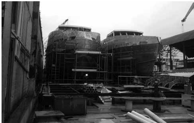
Two of twelve 48 m monohull UT4000 FSVs under construction at ETP Engenharia (Photo courtesy Incat Crowther)
