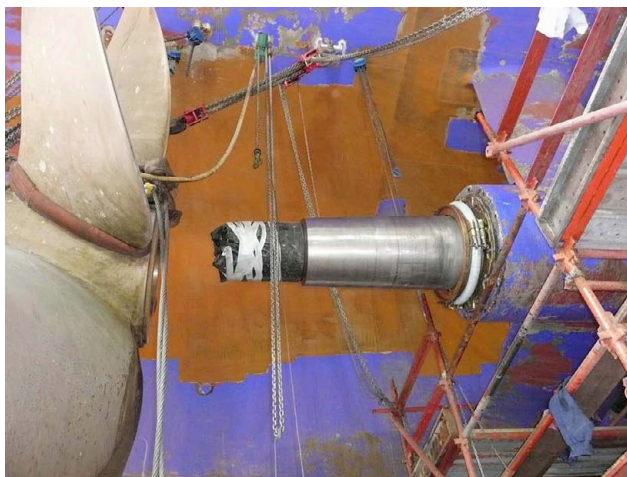
Propeller removal (Photo courtesy Carnival Australia)
