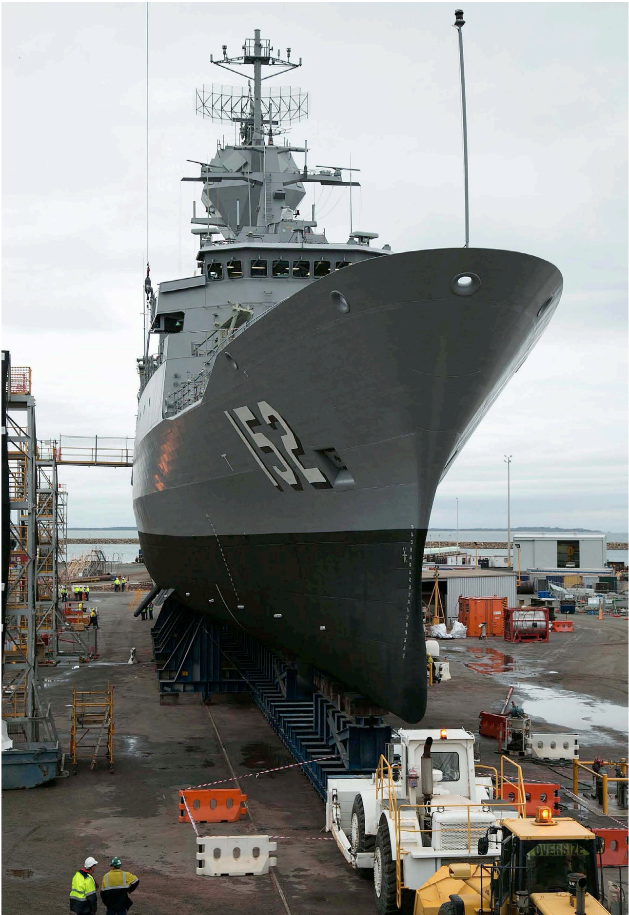
HMAS Warramunga about to be moved to the shiplift for undocking on 9 April after her anti-ship missile defence upgrade by BAE Systems at Henderson, Western Australia. Warramunga is the first RAN ship to be painted the RAN's new haze grey colour (RAN photograph)
