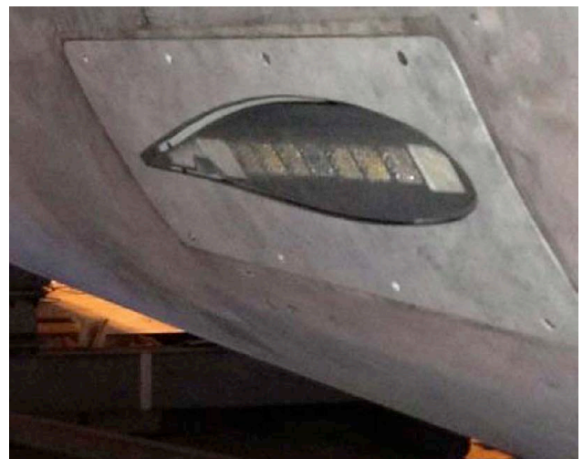
Hull plate for side lifting foil on Wild Oats XI (Photo courtesy Composites Consulting Group)
