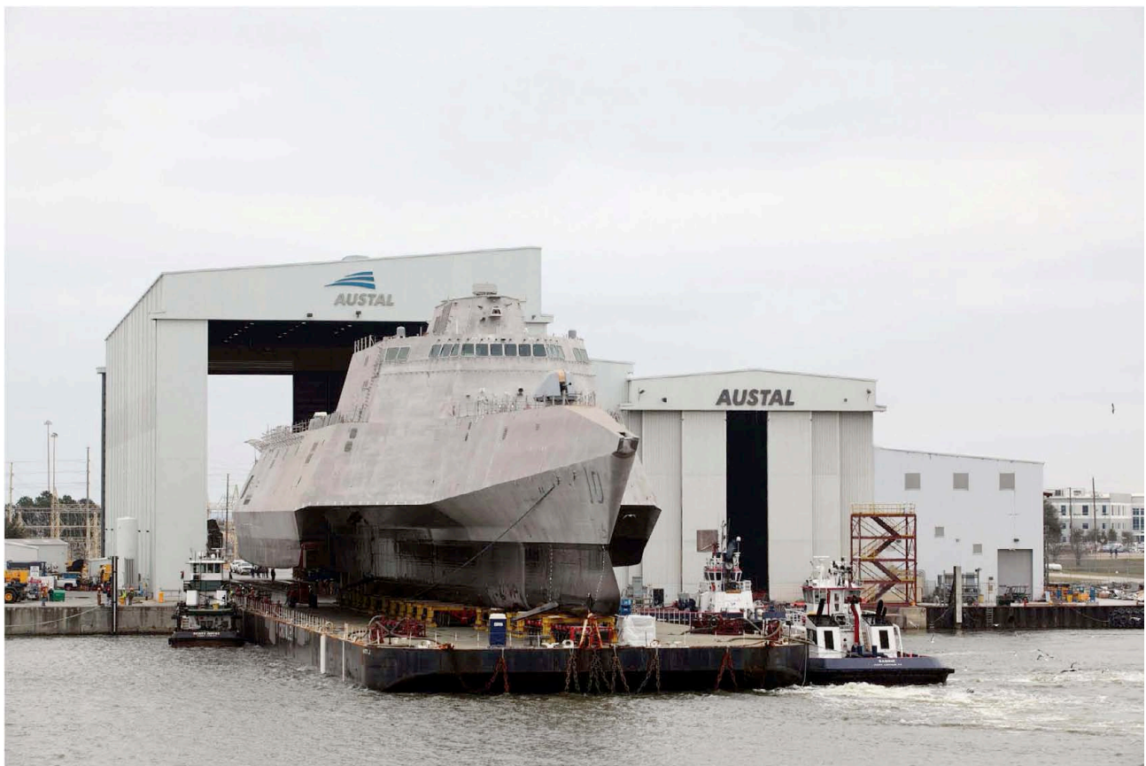
The future USS Gabrielle Giffords (LCS10) being transferred to a barge for launching at BAE Systems floating dock (Photo courtesy Austal)
