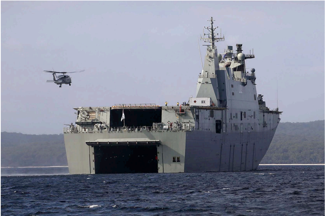
HMAS Canberra docked down with her stern door down to receive landing craft as a helicopter approaches the ship to land on deck during trials in Jervis Bay during March 2015 (RAN photograph)
