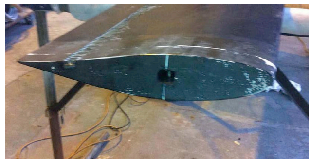
Construction of side lifting foil on Wild Oats XI (Photo courtesy Composites Consulting Group)
